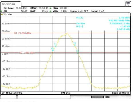
450.0125 MHz, 99% Occupied & 26 dB Bandwidth with Low Power
