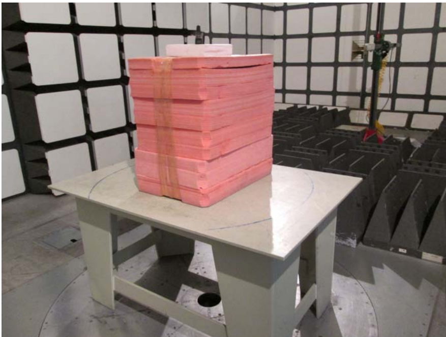
Transmitting Radiated Emissions View (Above 1 GHz)
