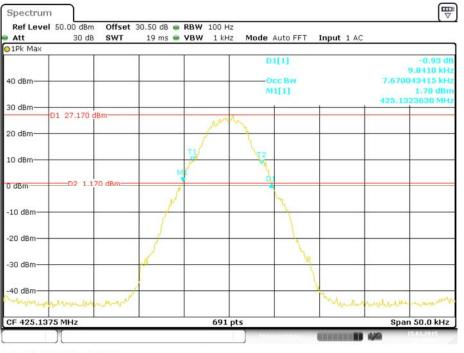
425.1375 MHz, 99% Occupied & 26 dB Bandwidth with Low Power
