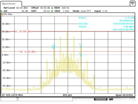
425.1375 MHz, 99% Occupied & 26 dB Bandwidth with Low Power
