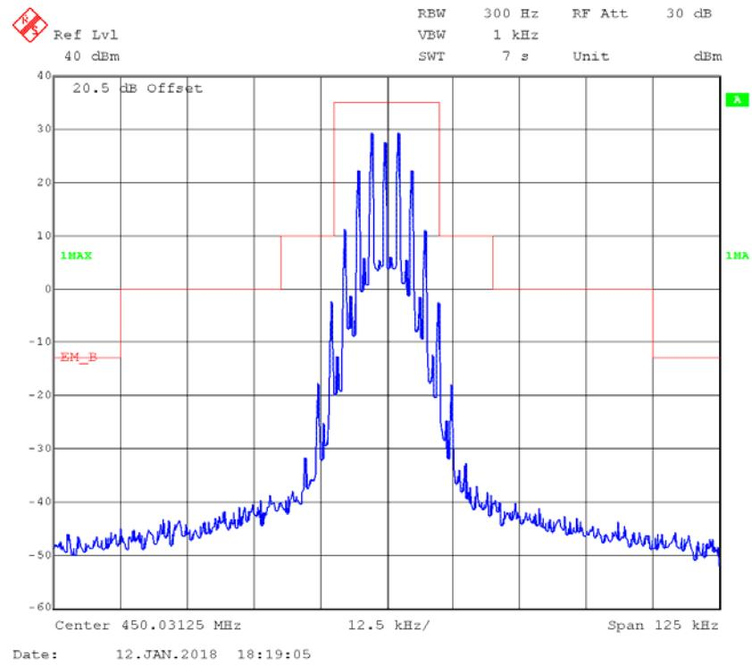
**FM,25kHz,Low Power - Frequency 450.03125 MHz: 99% Occupied & 26 dB Bandwidth**
