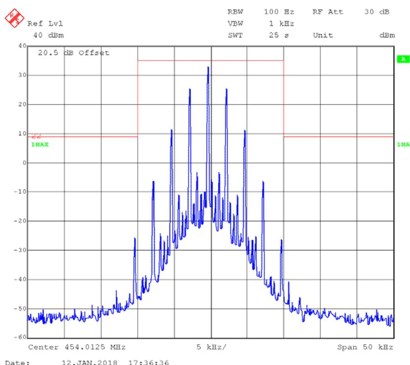
**FM,25kHz,Low Power - Frequency 454.0125 MHz: 99% Occupied & 26 dB Bandwidth**
