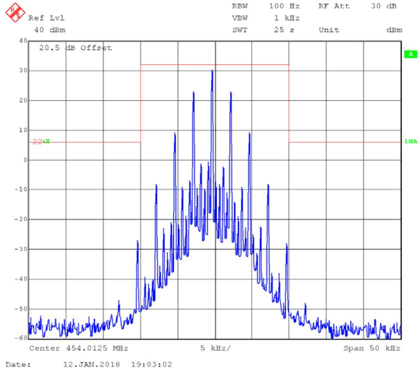
**FM,25kHz,High Power - Frequency 454.0125 MHz: 99% Occupied & 26 dB Bandwidth**
