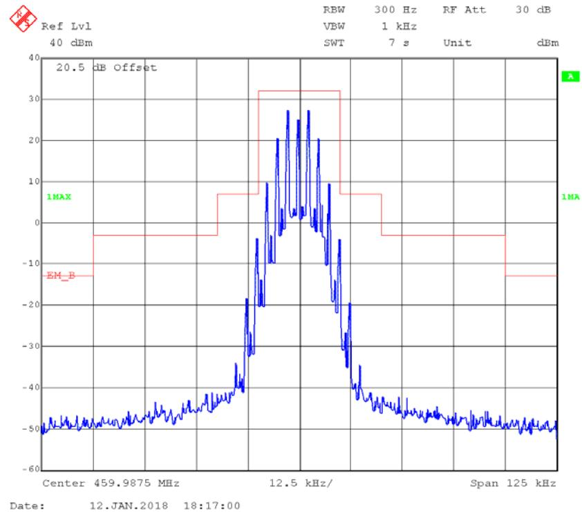
**Part 74****FM,12.5kHz,High Power - Frequency 450.03125 MHz: 99% Occupied & 26 dB Bandwidth**
