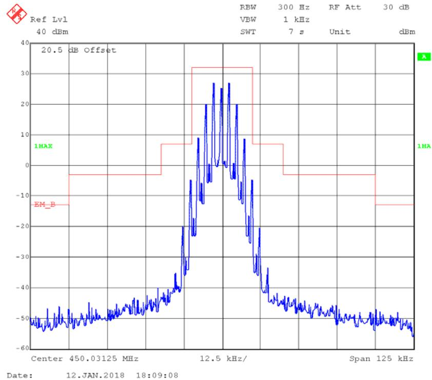
**4FSK,12.5kHz,High Power - Frequency 450.03125 MHz: 99% Occupied & 26 dB Bandwidth**
