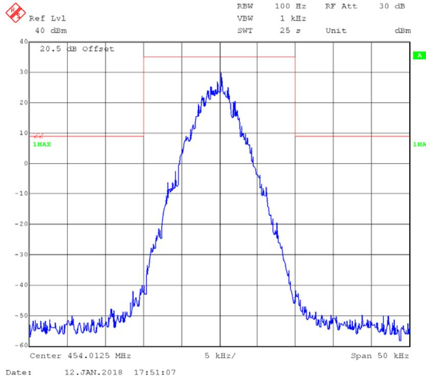
**4FSK,12.5kHz,Low Power - Frequency 454.0125 MHz: 99% Occupied & 26 dB Bandwidth**
