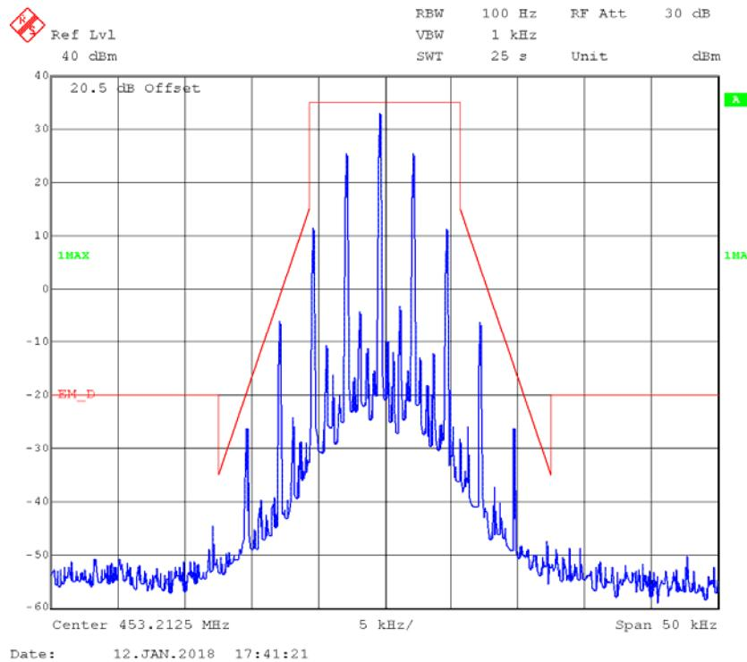
**FM,12.5kHz,Low Power - Frequency 453.2125 MHz: 99% Occupied & 26 dB Bandwidth**
