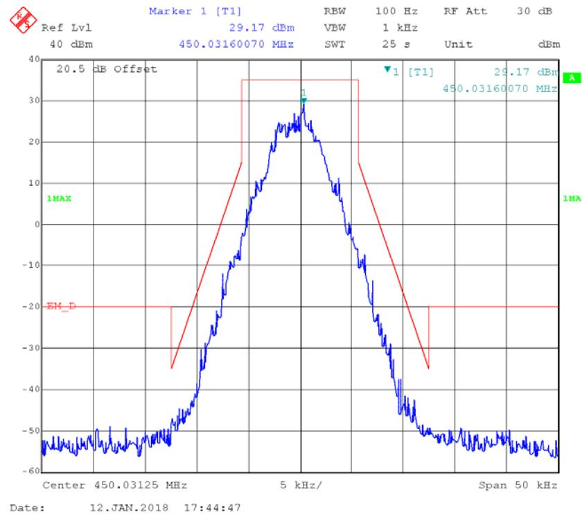
**4FSK,12.5kHz,Low Power - Frequency 450.03125 MHz: 99% Occupied & 26 dB Bandwidth**
