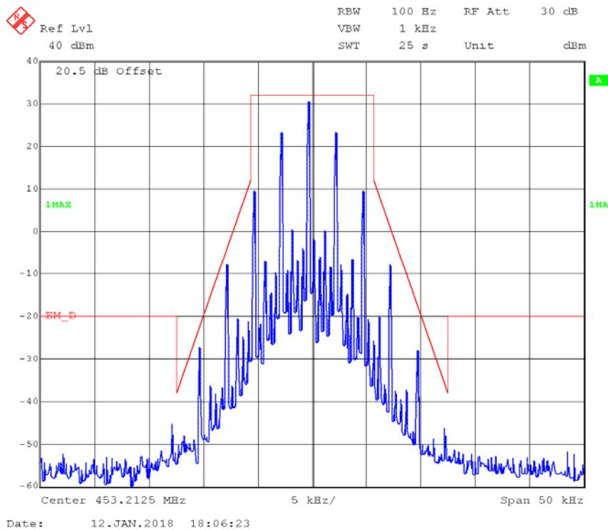
**4FSK,12.5kHz,High Power - Frequency 453.2125 MHz: 99% Occupied & 26 dB Bandwidth**
