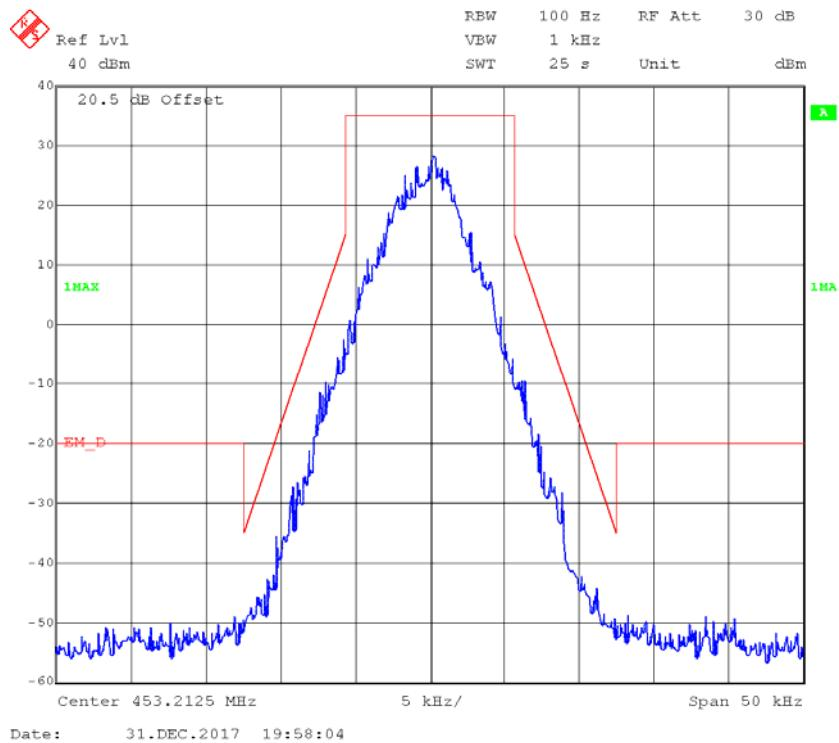
**4FSK,12.5kHz,Low Power - Frequency 453.2125 MHz: 99% Occupied & 26 dB Bandwidth**
