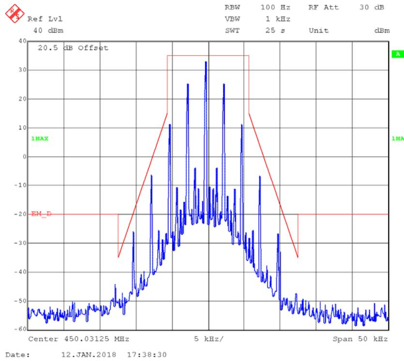
**FM,12.5kHz,Low Power - Frequency 450.03125 MHz: 99% Occupied & 26 dB Bandwidth**
