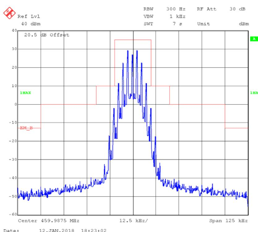
**FM,25kHz,Low Power - Frequency 459.9875 MHz MHz: 99% Occupied & 26 dB Bandwidth**
