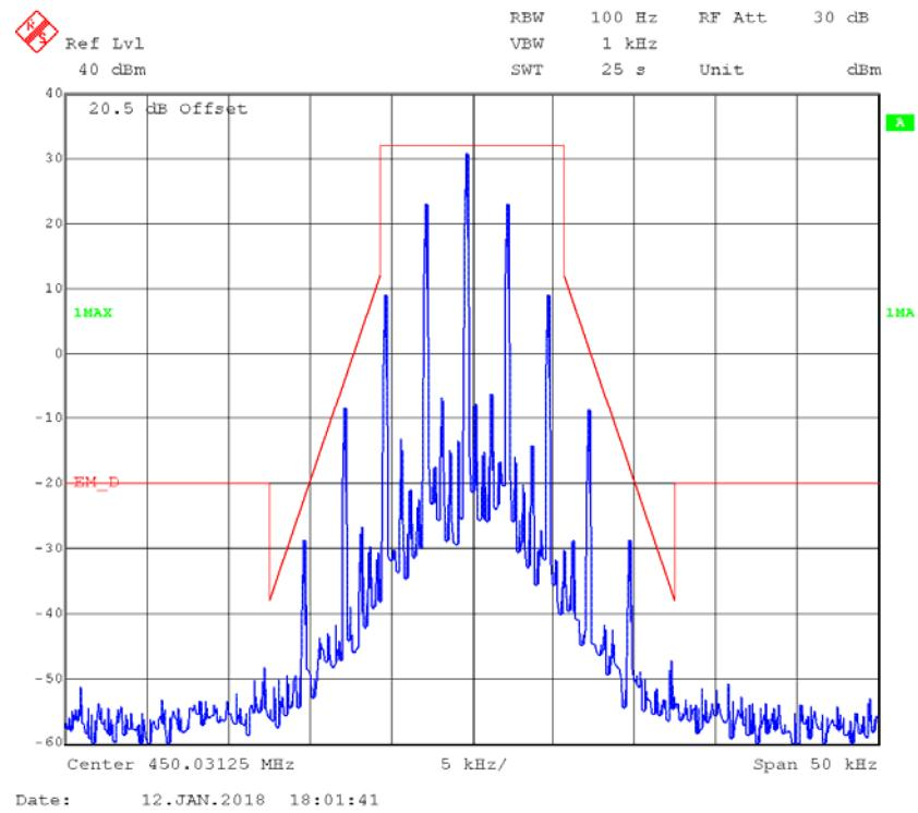
**FM,25kHz,High Power - Frequency 450.03125 MHz: 99% Occupied & 26 dB Bandwidth**
