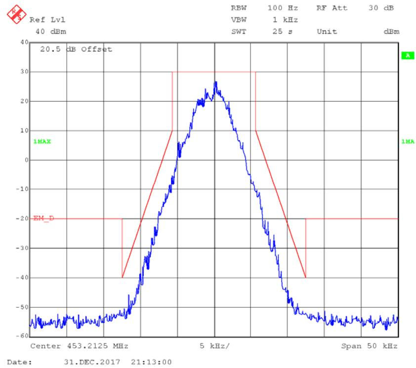
**Part 80:****FM,25kHz,High Power - Frequency 459.9875 MHz MHz: 99% Occupied & 26 dB Bandwidth**
