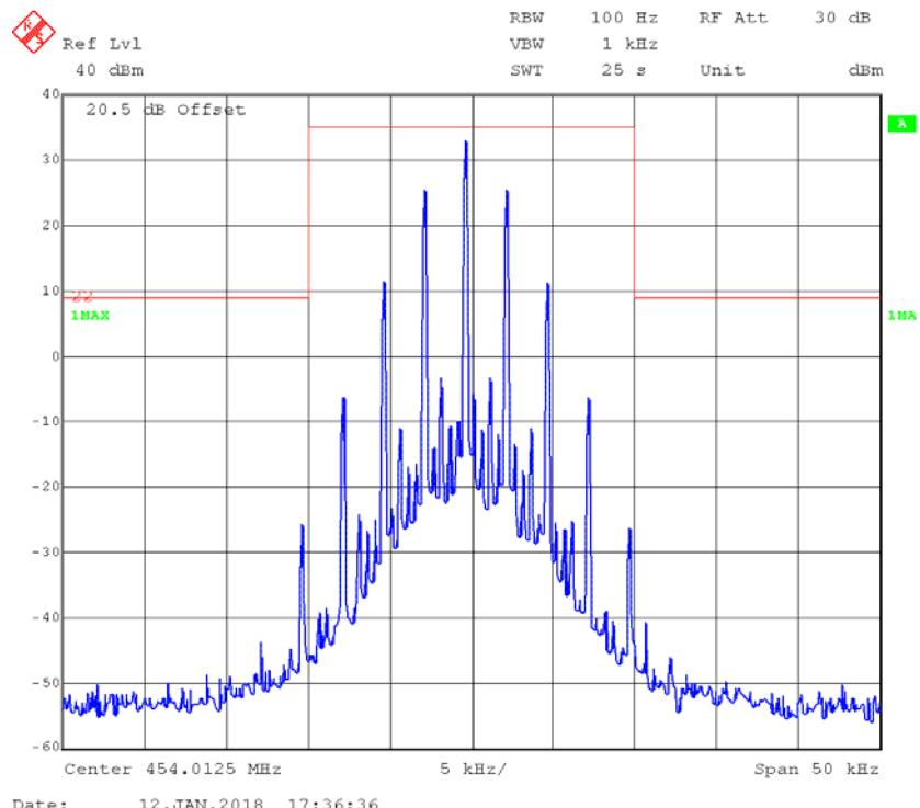
**FM,12.5kHz,Low Power - Frequency 454.0125 MHz: 99% Occupied & 26 dB Bandwidth**
