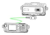
**Step 4** Connect the accessories following Step 4 for installation of mobile terminal.
