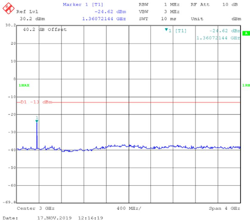
**4FSK,12.5kHz,High Power - Frequency 454.0125 MHz**
