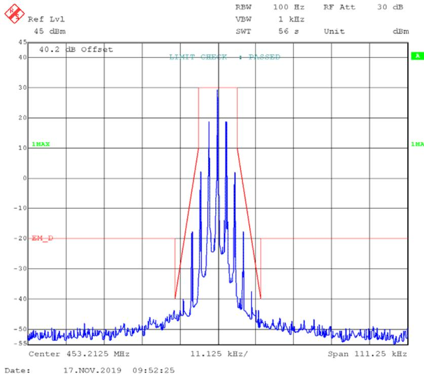
**4FSK,12.5kHz,High Power - Frequency 453.2125 MHz:**
