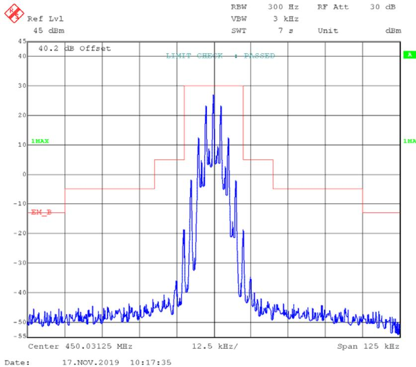
**4FSK,12.5kHz,High Power - Frequency 450.03125 MHz:**
