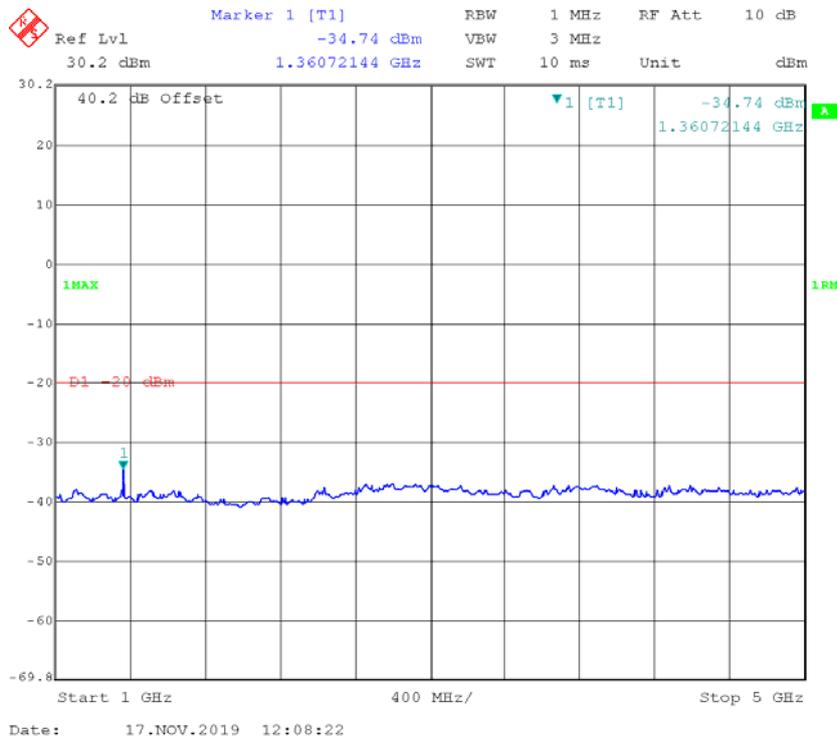
**4FSK,12.5kHz,High Power - Frequency 453.2125 MHz**
