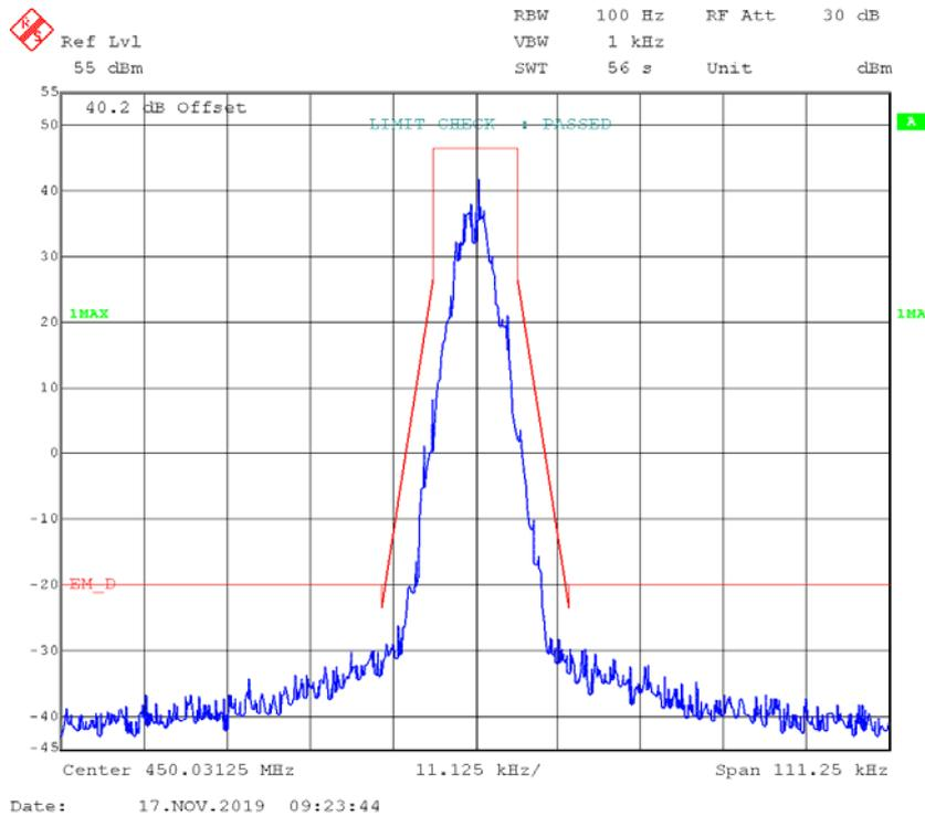
**4FSK,12.5kHz,Low Power - Frequency 450.03125 MHz:**
