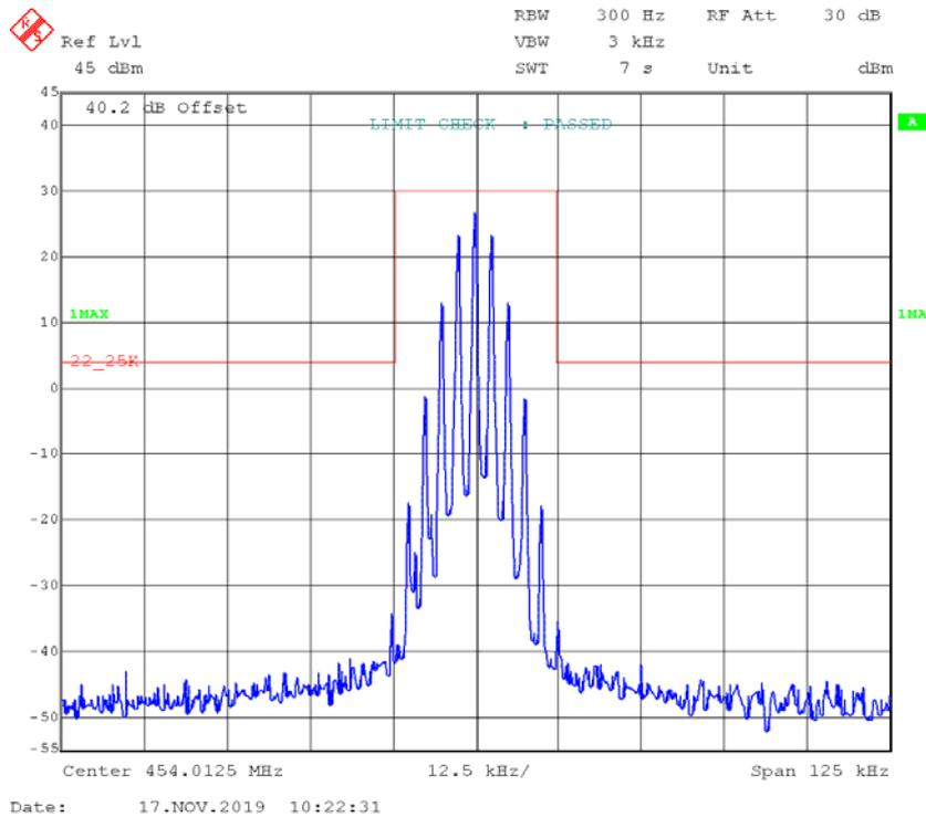
**4FSK,12.5kHz,High Power - Frequency 454.0125 MHz:**
