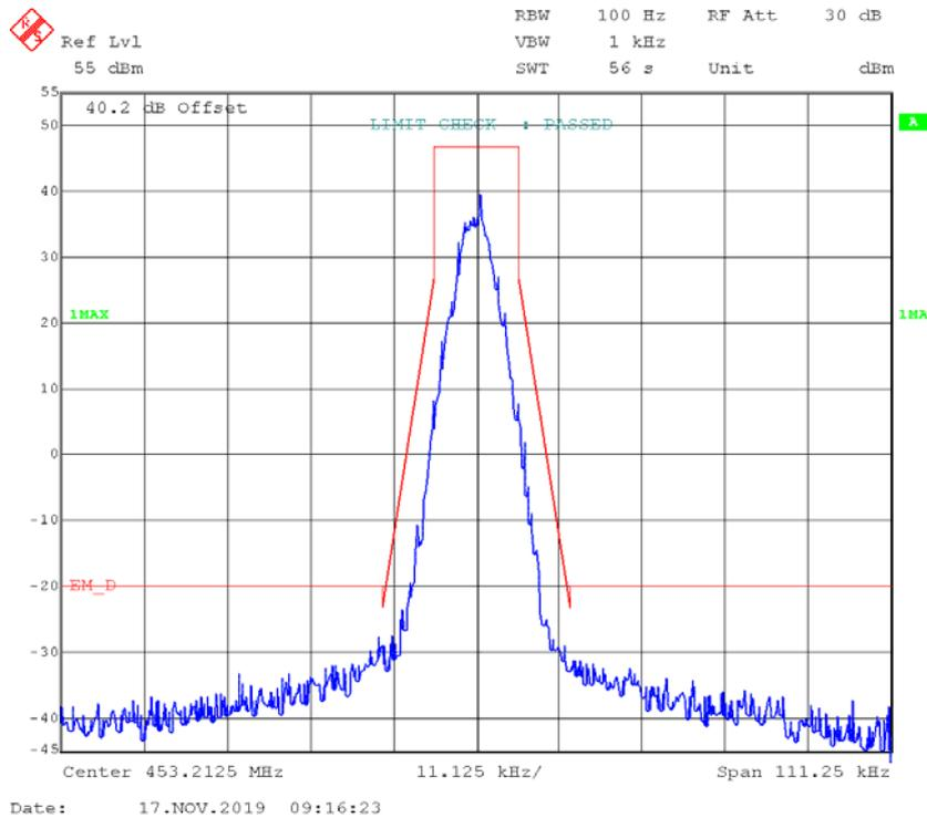
**4FSK,12.5kHz,Low Power - Frequency 453.2125 MHz:**
