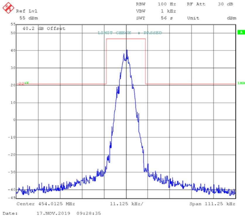
**4FSK,12.5kHz,Low Power - Frequency 454.0125 MHz:**
