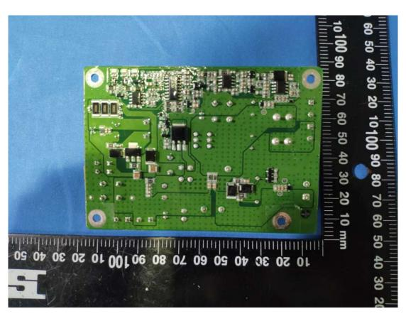
Network Board (Double Ethernet Interface Configuration)
