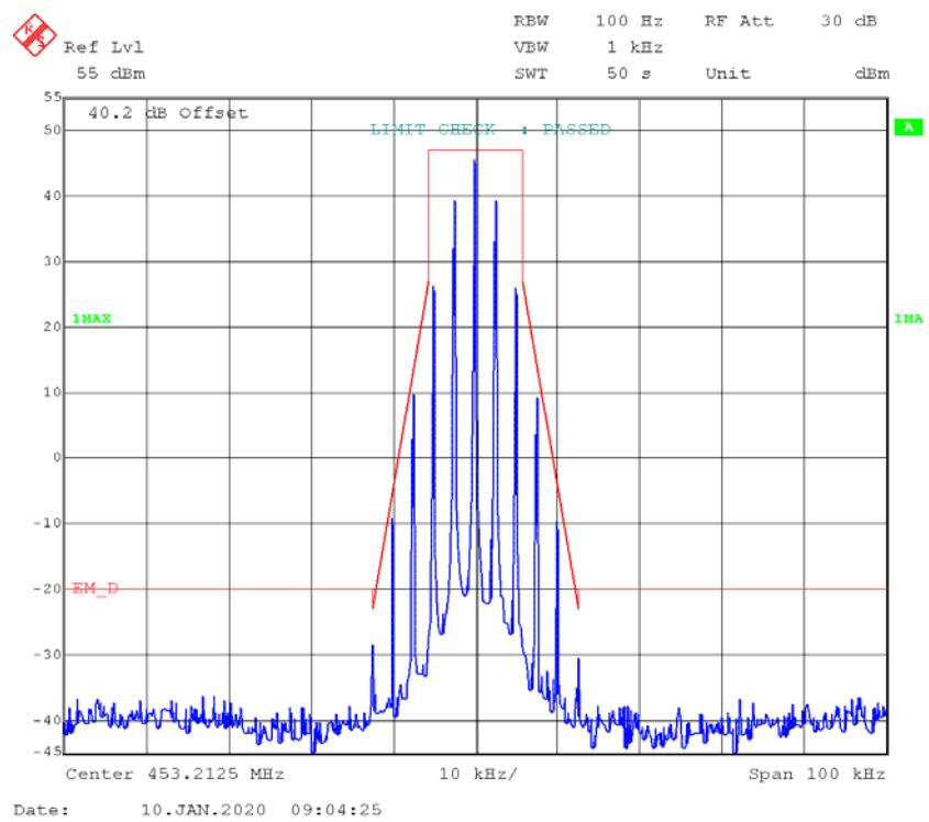
**FM,12.5kHz,Low Power - Frequency 453.2125 MHz:****99% Occupied & 26 dB Bandwidth**
