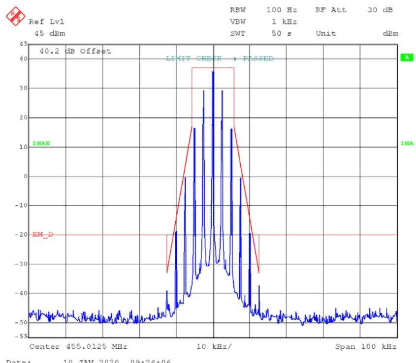
**FM,25kHz,High Power - Frequency 455.0125 MHz****99% Occupied & 26 dB Bandwidth**
