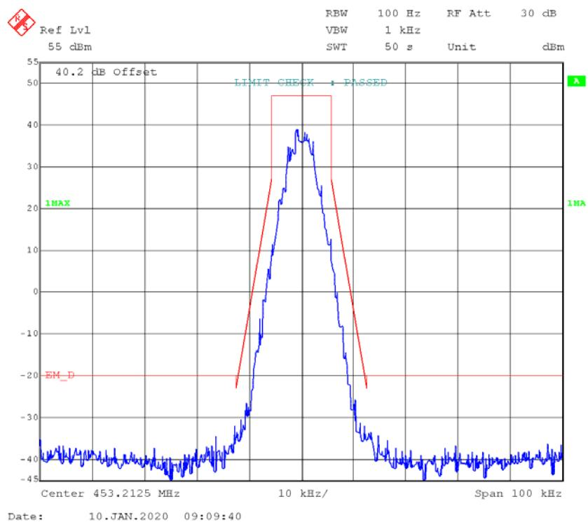
**4FSK,12.5kHz,Low Power - Frequency 453.2125 MHz:****99% Occupied & 26 dB Bandwidth**
