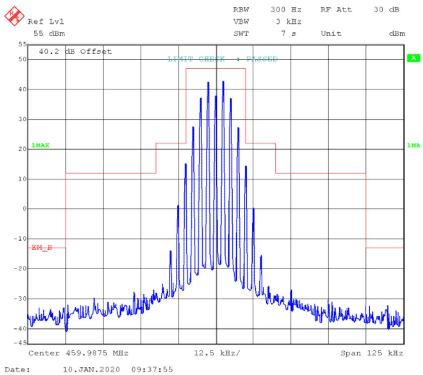
**FM,25kHz,Low Power - Frequency 459.9875 MHz:****99% Occupied & 26 dB Bandwidth**
