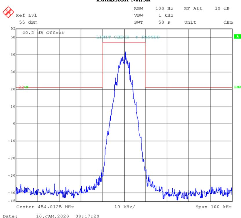
**4FSK,12.5kHz,Low Power - Frequency 454.0125MHz:****99% Occupied & 26 dB Bandwidth**
