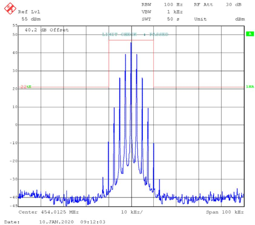
**FM,12.5kHz,Low Power - Frequency 454.0125MHz:****99% Occupied & 26 dB Bandwidth**
