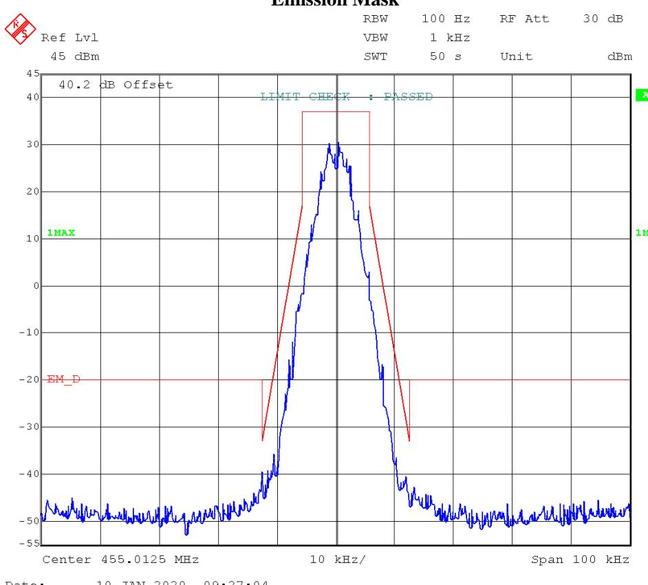
**4FSK ,12.5kHz, High Power - Frequency 455.0125 MHz:****99% Occupied & 26 dB Bandwidth**
