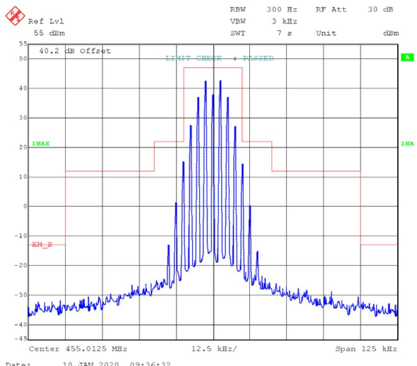
**FM,25kHz,Low Power - Frequency 455.0125 MHz:****99% Occupied & 26 dB Bandwidth**
