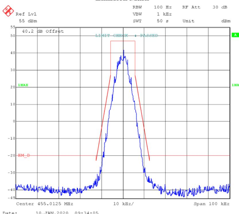
**4FSK ,12.5kHz, Low Power - Frequency455.0125 MHz:****99% Occupied & 26 dB Bandwidth**
