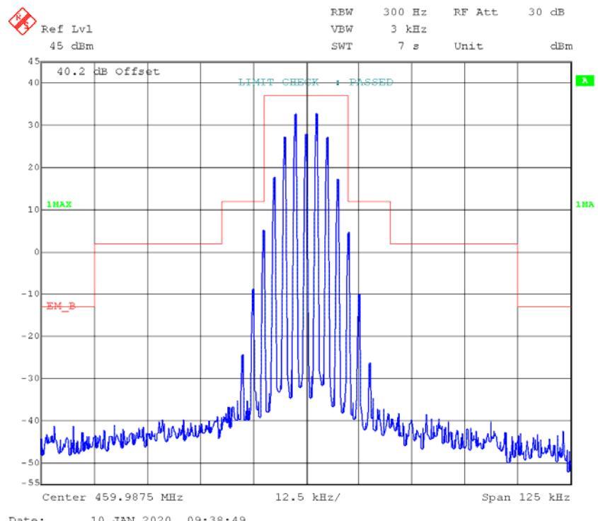
**part 74:****FM,12.5kHz,High Power - Frequency 455.0125 MHz:****99% Occupied & 26 dB Bandwidth**
