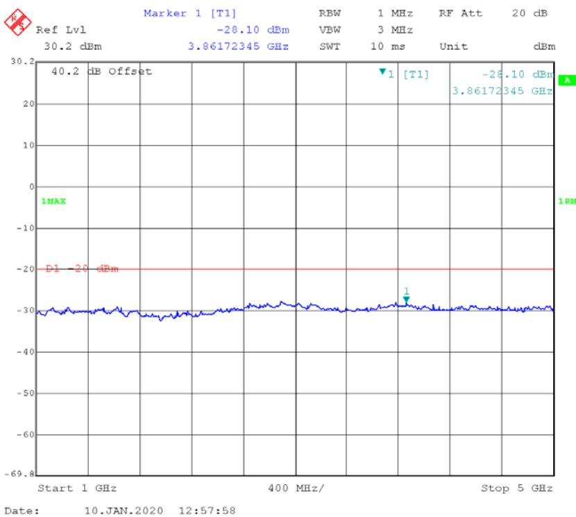
**12.5kHz,4FSK, High power, 453.2125 MHz**
