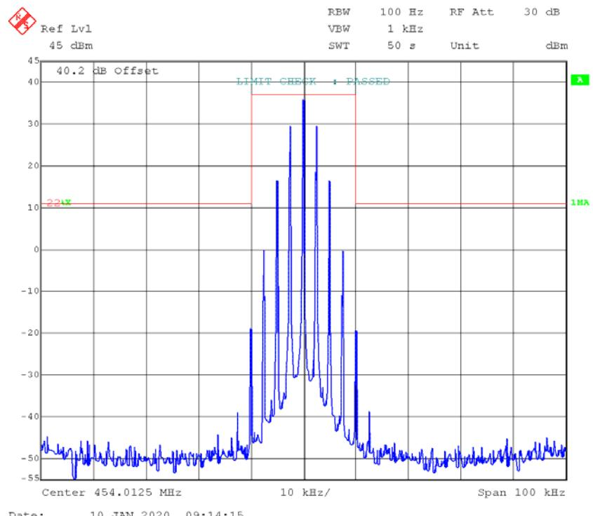
**FM,25kHz,High Power - Frequency 454.0125 MHz:****99% Occupied & 26 dB Bandwidth**
