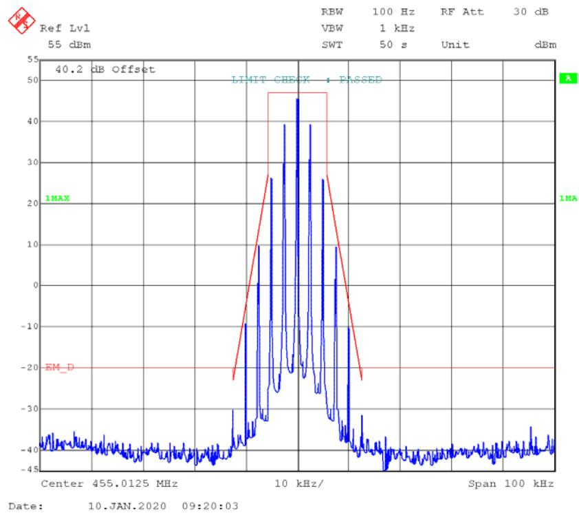
**FM,12.5kHz,Low Power – Frequency 455.0125 MHz:****99% Occupied & 26 dB Bandwidth**
