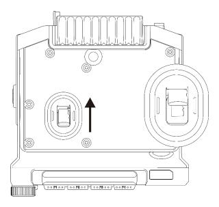
4. Align the concave side of the plastic upper cover with the aluminum chassis, and then press the cover until the latches are properly locked.
