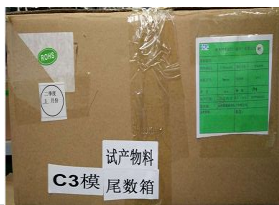
Figure 5: The upper right-hand corner affixed with ready-made tickets, the upper left-hand corner affixed with Rohs and month labels, the lower left-hand corner affixed with status label model number, etc. .
