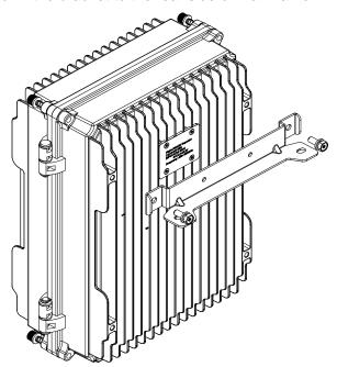
2. Use four M6x16 bolts to fix the pole-mounted bracket to the pole-mounted bracket components.
