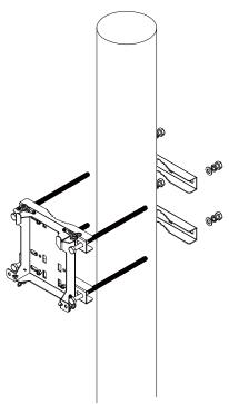
5. Adopt the same method to install antenna bracket components, GPS antenna, Bei Dou antenna and RF antenna.
