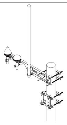
6. Fix the bracket of mainframe to pole-mounted bracket components with four M6×16 bolts ①.
