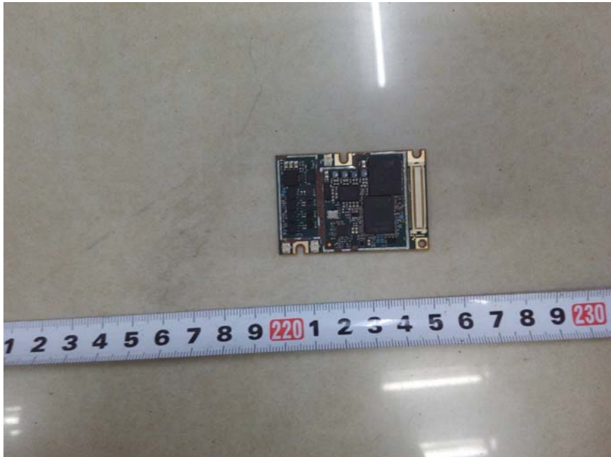
EUT – RF Module Bottom Shielding off View
