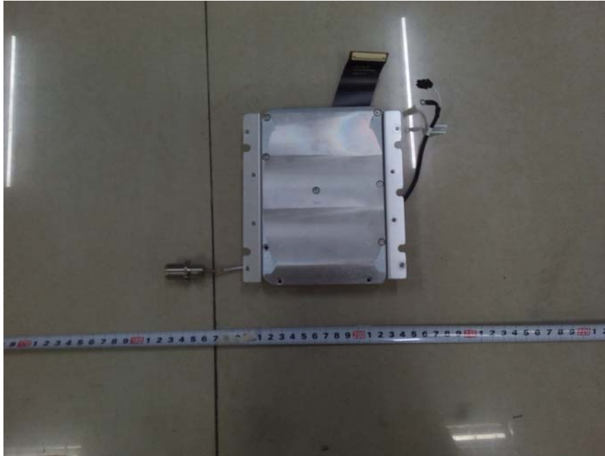
EUT – Amplifier Front View
