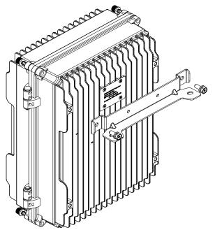
2. Use four M6×16 bolts to fix the pole-mounted bracket to the pole-mounted bracket components.
