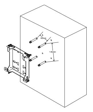
5. Fix bracket of the mainframe to the wall-mounted components, and use four M6x16 bolts ① to fix it.
