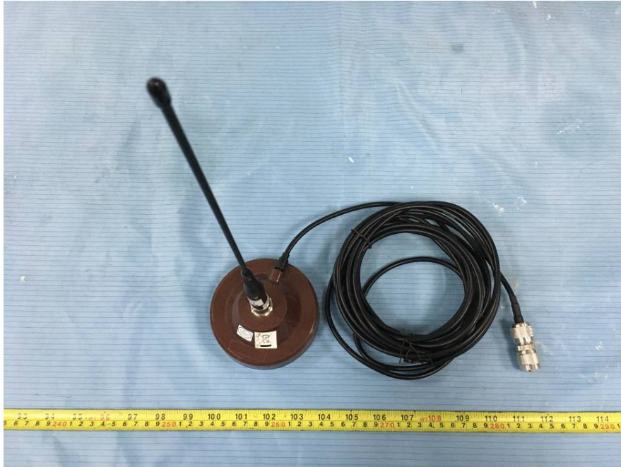
EUT – DMR Antenna View
