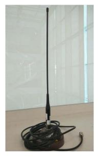
The threaded end of sucker antenna should be inserted in the RF interface at the top of the host, and then screw it in clockwise direction.
