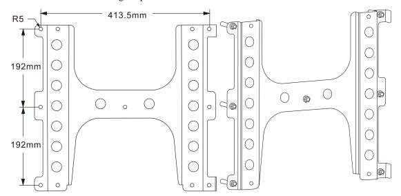
2. Align the hang holes on the back of the main EDS50 with the protrusions on the bracket.
