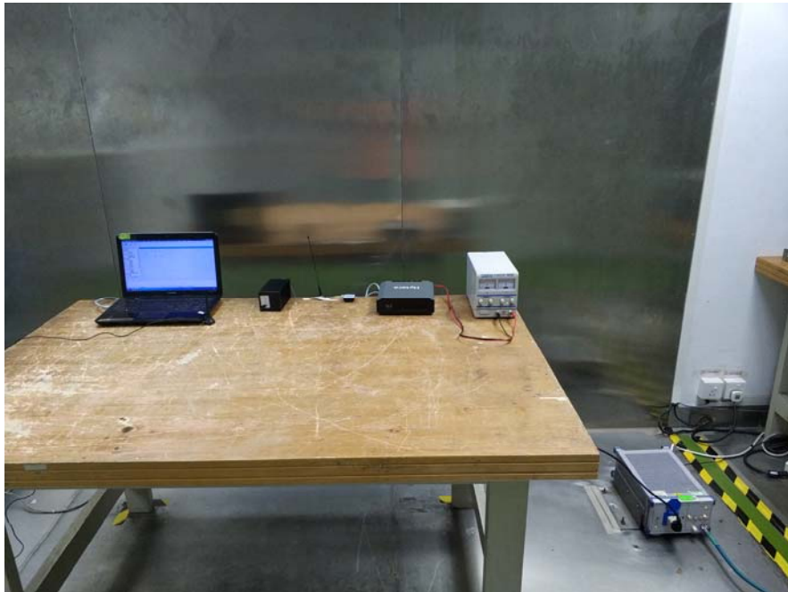
Conducted Emissions - Front View
