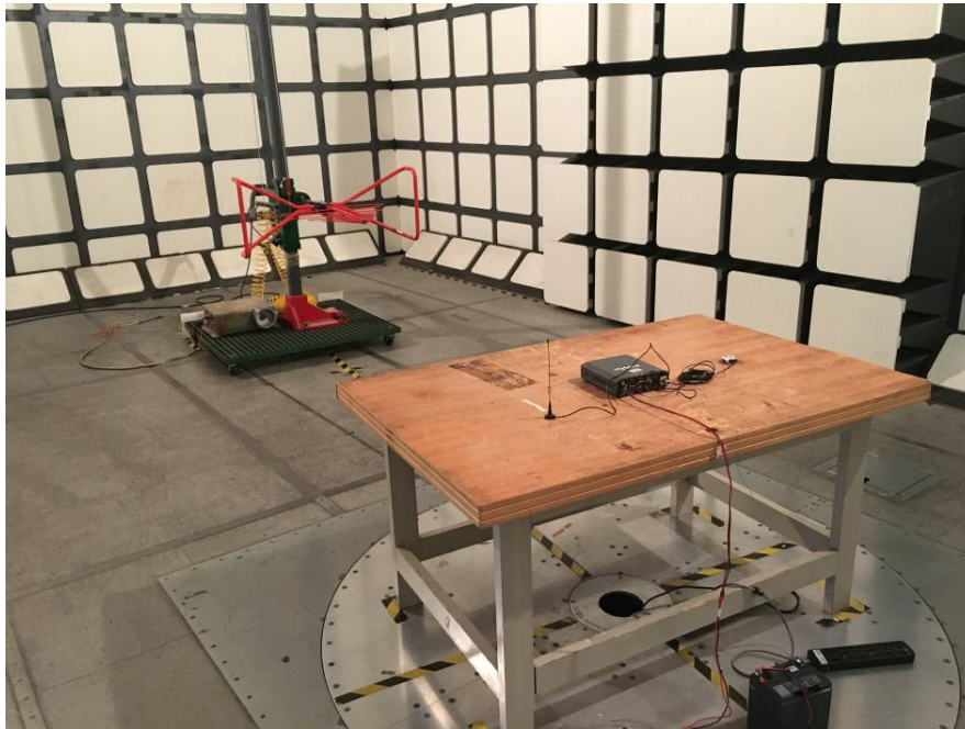
Radiated Emissions View (Below 1 GHz)
