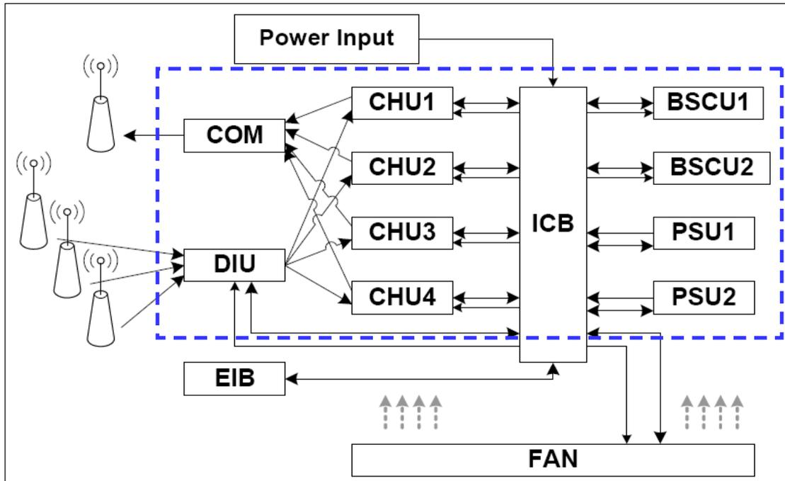
After going through the antenna, the service signal reaches DIU and CHU, where the signal will be delivered to baseband after appropriate processing. Then the baseband will send the service signal to BSCU for soft switch. Afterwards, the signal will be sent back via ICB to baseband, which would convert it into HF signal and send it to the transmitter. Finally, the transmitter will deliver the HF service signal to antenna via COM.
