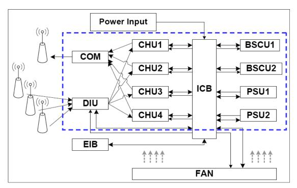
After going through the antenna, the service signal reaches DIU and CHU, where the signal will be delivered to baseband after appropriate processing. Then the baseband will send the service signal to BSCU for soft switch. Afterwards, the signal will be sent back via ICB to baseband, which would convert it into HF signal and send it to the transmitter. Finally, the transmitter will deliver the HF service signal to antenna via COM.
