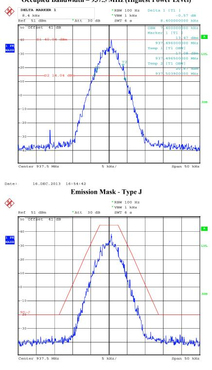
Occupied Bandwidth - 937.5 MHz (Highest Power Level)
