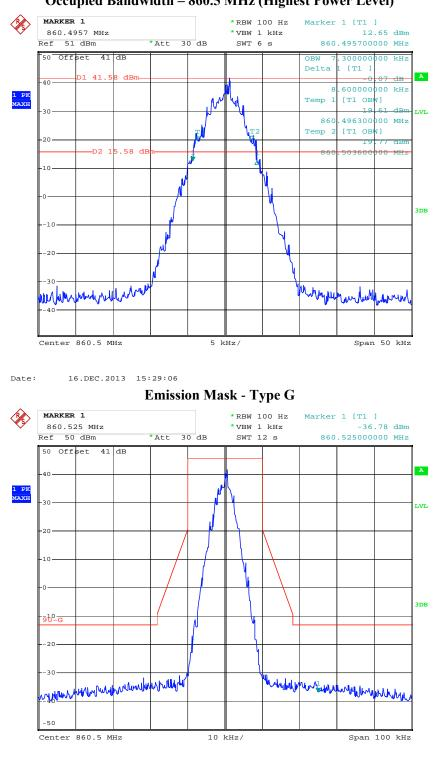
Occupied Bandwidth - 860.5 MHz (Highest Power Level)
