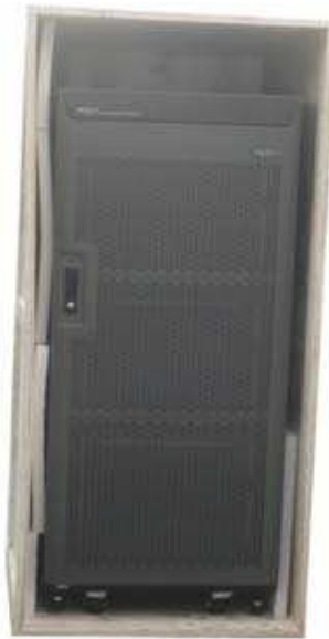
Figure 3-3 Erecting the Wooden Case
