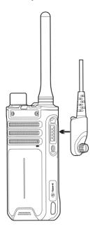
3. Tighten the screw on the audio accessory plug.
