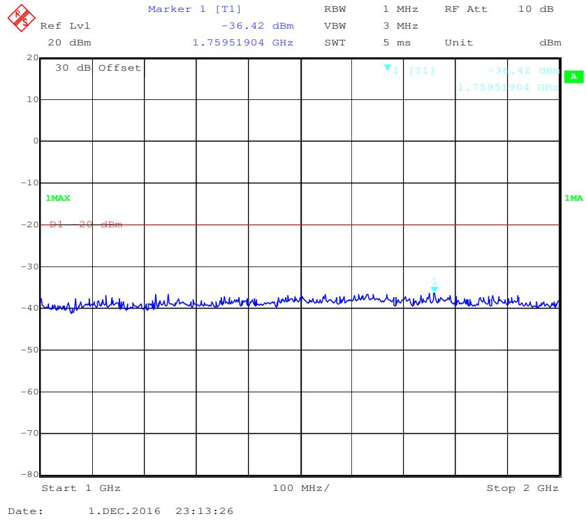
**30MHz - 1 GHz, 158.55 MHz—part 22**
