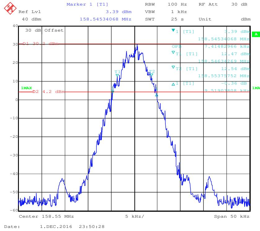
**Frequency 158.55 MHz: 99% Occupied & 26 dB Bandwidth with Low Power**
