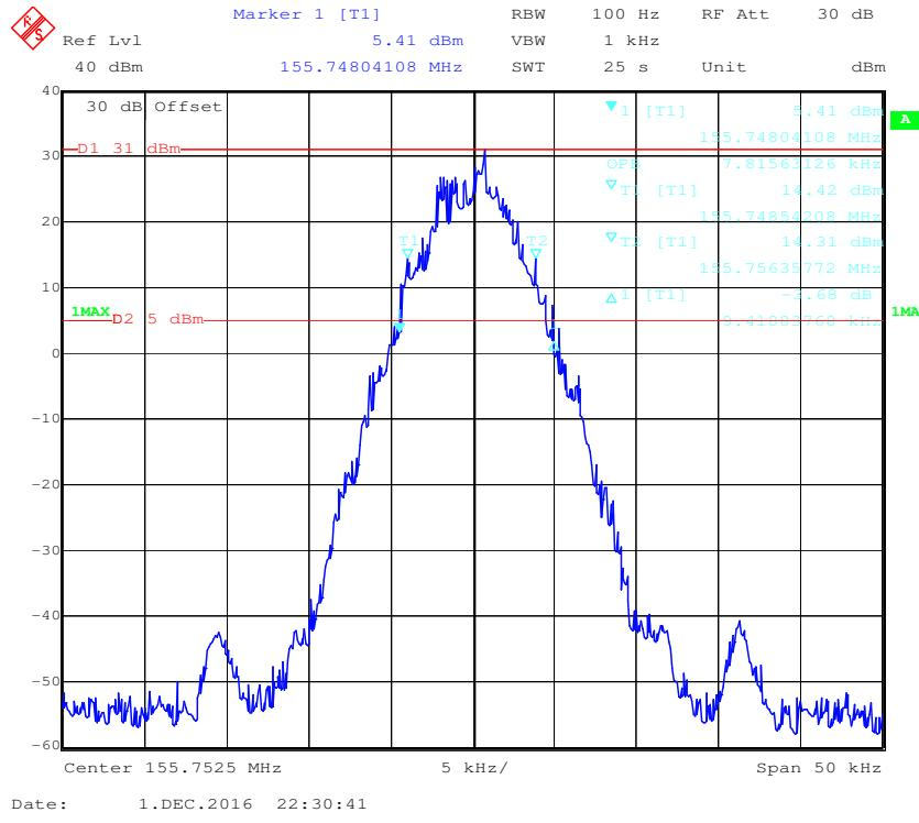
**Frequency 155.7525 MHz: 99% Occupied & 26 dB Bandwidth with Low Power**
