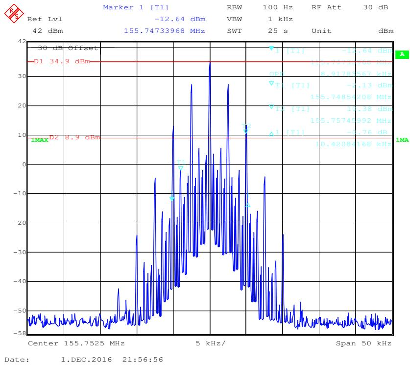
**Frequency 155.7525 MHz: 99% Occupied & 26 dB Bandwidth, Low Power**
