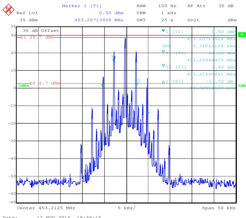
**Frequency 454.0125 MHz: 99% Occupied & 26 dB Bandwidth, High Power**
