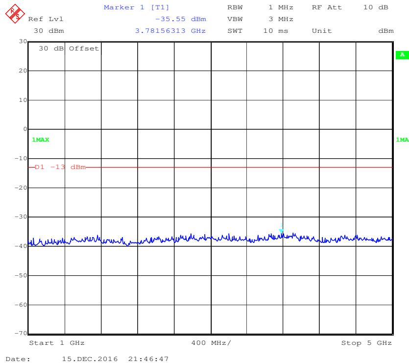
**Digital Modulation:****30MHz - 1 GHz, 453.2125MHz – PART 90**
