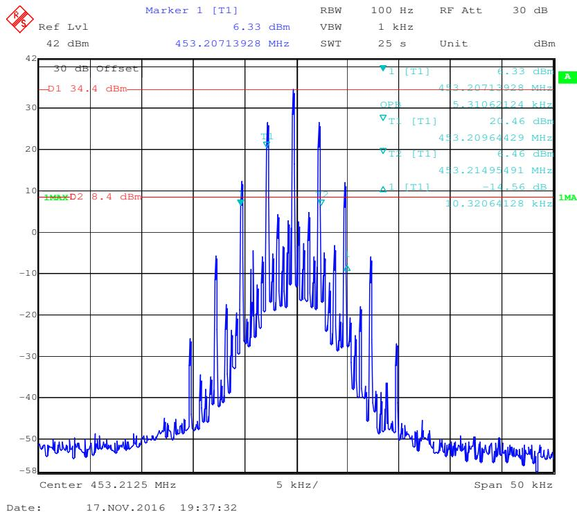
**Frequency 453.2125 MHz: 99% Occupied & 26 dB Bandwidth, Low Power**
