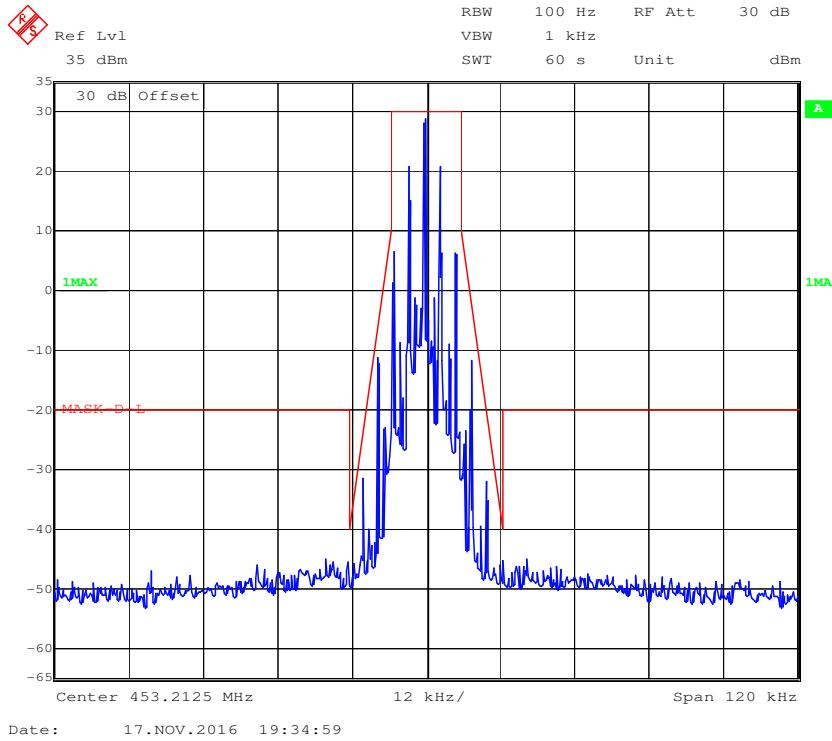
**Digital Modulation:****Frequency 453.2125 MHz: 99% Occupied & 26 dB Bandwidth, High Power**
