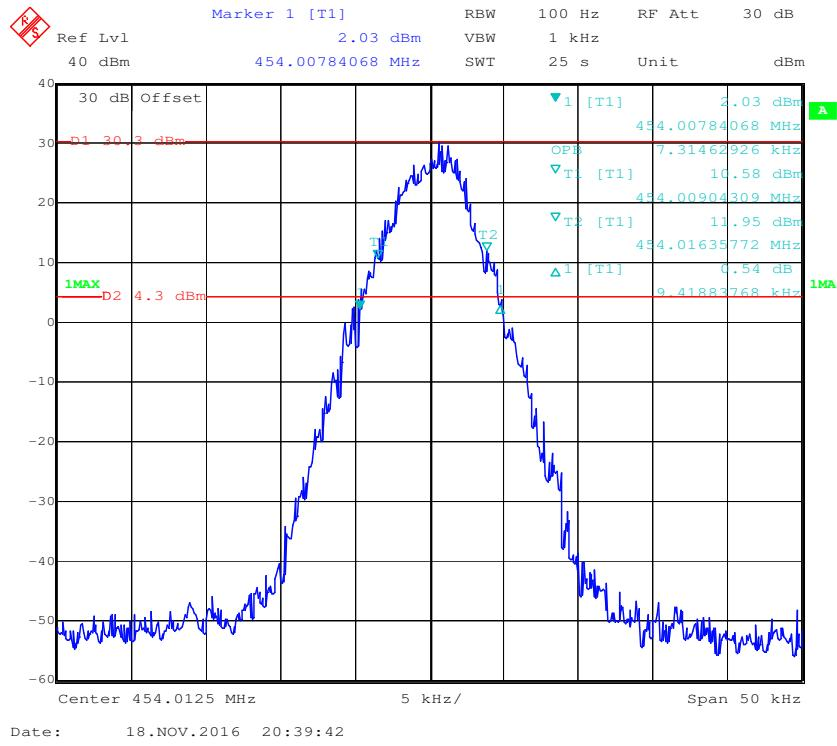
**Frequency 454.0125 MHz: 99% Occupied & 26 dB Bandwidth, Low Power**
