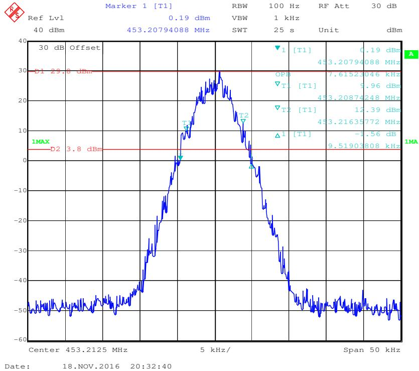
**Frequency 453.2125 MHz: 99% Occupied & 26 dB Bandwidth, Low Power**
