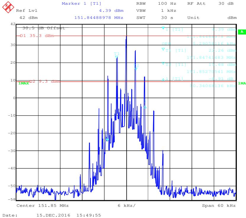
**Frequency 151.85 MHz: 99% Occupied & 26 dB Bandwidth, Low Power**
