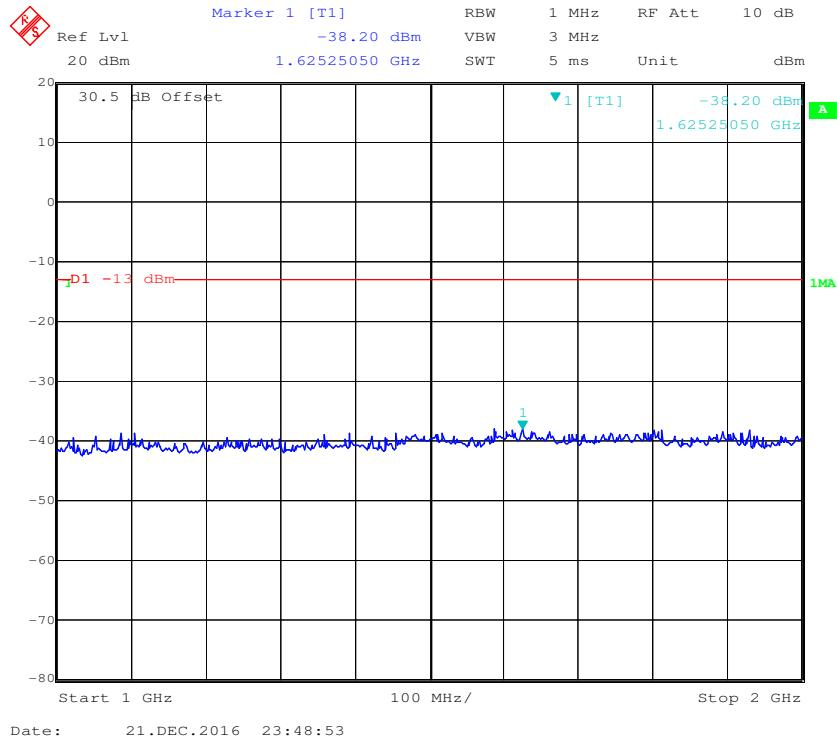
**30MHz - 1 GHz, 155.7525MHz, For Part 90**
