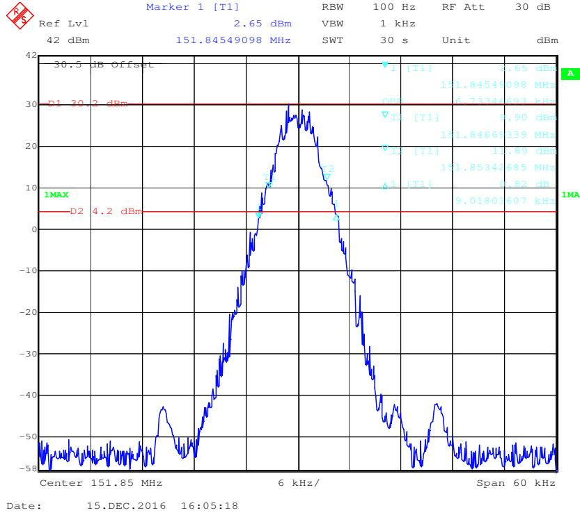
**Frequency 151.85 MHz: 99% Occupied & 26 dB Bandwidth, Low Power**
