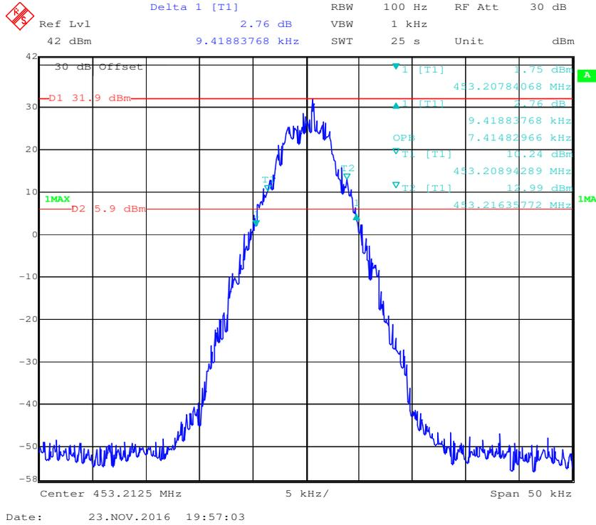
**Frequency 453.2125 MHz: 99% Occupied & 26 dB Bandwidth, Low Power**
