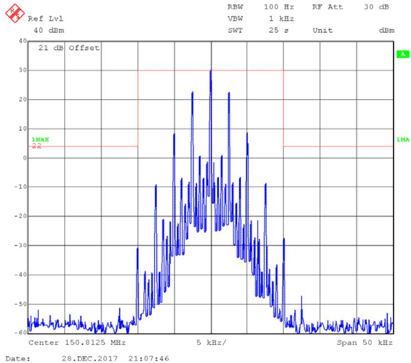
**FM,25kHz,High Power - Frequency 150.8125 MHz: 99% Occupied & 26 dB Bandwidth**
