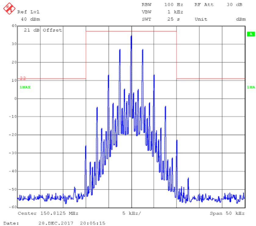
**FM,12.5kHz,Low Power - Frequency 150.8125 MHz: 99% Occupied & 26 dB Bandwidth**
