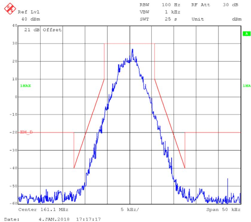
**Part 22****FM,12.5kHz,High Power - Frequency 150.8125 MHz: 99% Occupied & 26 dB Bandwidth**
