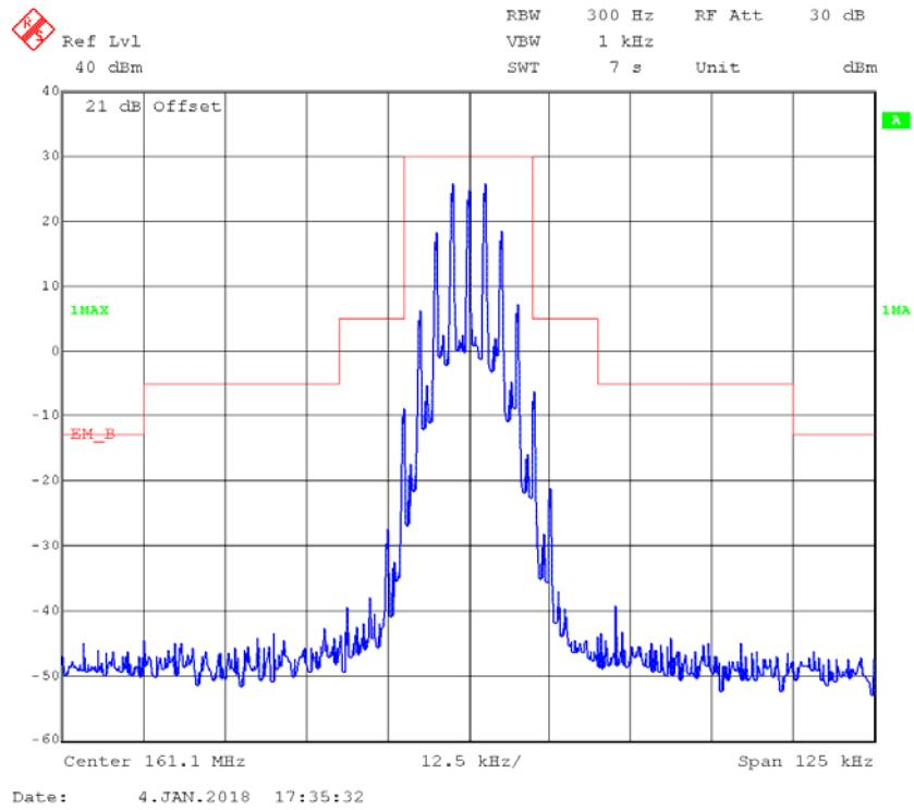
**4FSK,12.5kHz,High Power - Frequency 161.1 MHz: 99% Occupied & 26 dB Bandwidth**
