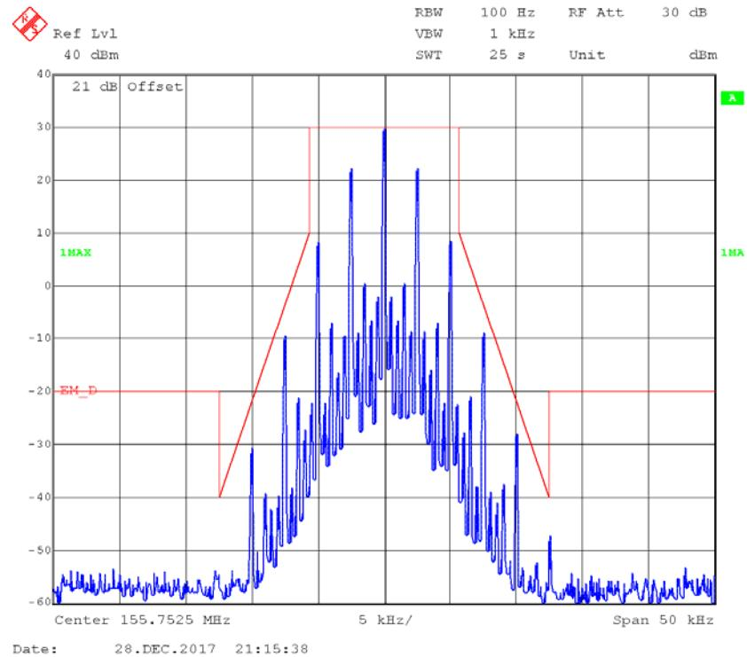
**4FSK,12.5kHz,High Power - Frequency 155.7525 MHz: 99% Occupied & 26 dB Bandwidth**
