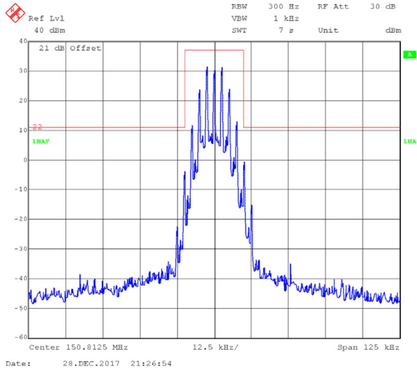
**FM,25kHz,Low Power - Frequency 150.8125 MHz: 99% Occupied & 26 dB Bandwidth**
