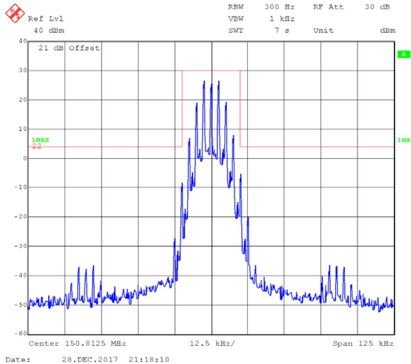
**4FSK,12.5kHz,High Power - Frequency 150.8125 MHz: 99% Occupied & 26 dB Bandwidth**
