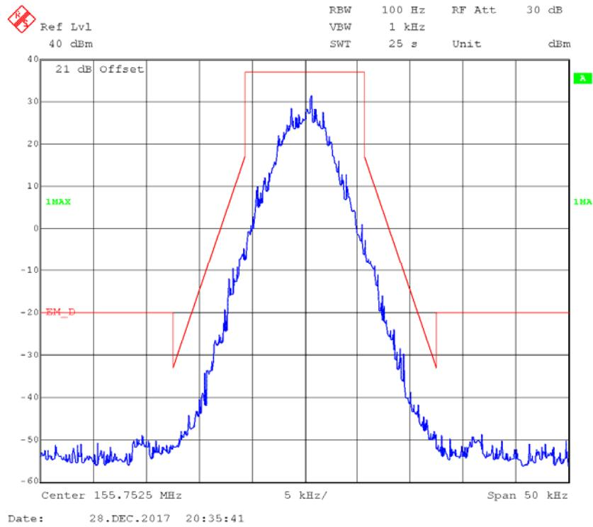
**4FSK,12.5kHz,Low Power - Frequency 155.7525 MHz: 99% Occupied & 26 dB Bandwidth**
