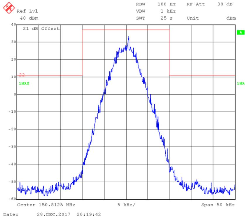
**4FSK,12.5kHz,Low Power - Frequency 150.8125 MHz: 99% Occupied & 26 dB Bandwidth**
