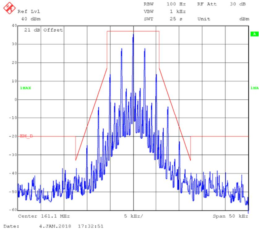
**FM,12.5kHz,Low Power - Frequency 161.1 MHz: 99% Occupied & 26 dB Bandwidth**
