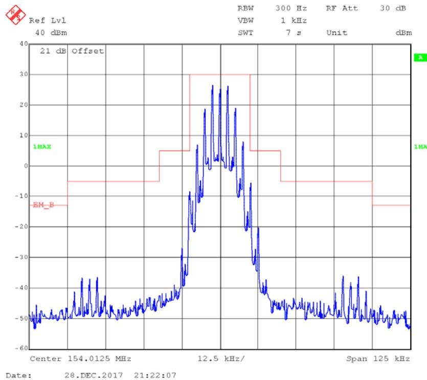
**Part 74****FM,12.5kHz,High Power - Frequency 161.1 MHz: 99% Occupied & 26 dB Bandwidth**
