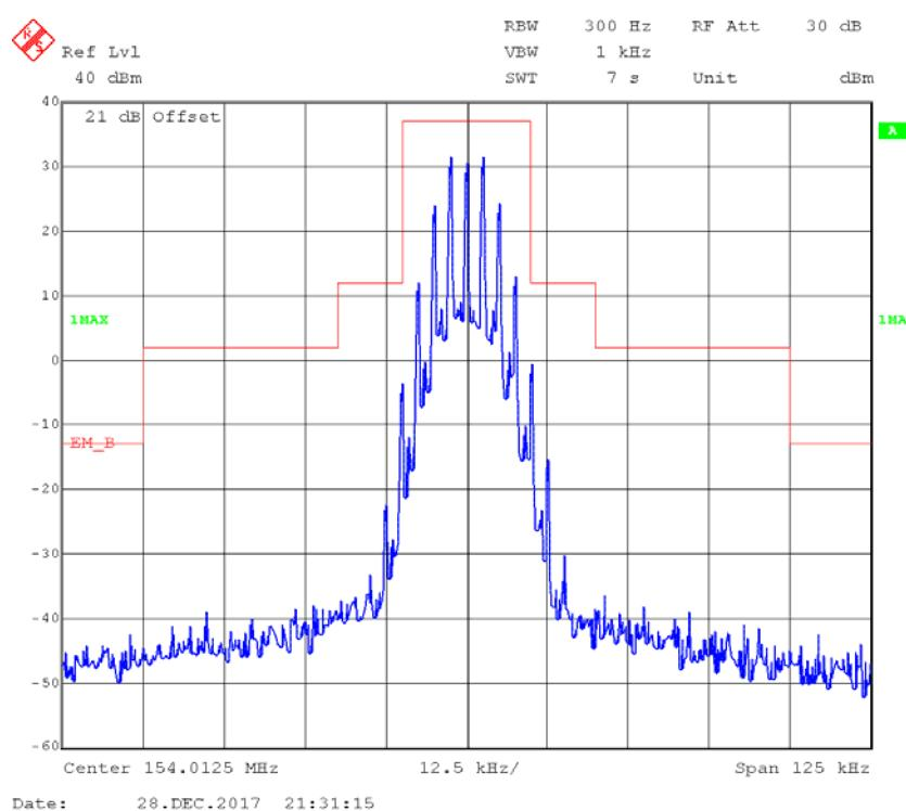
**FM,25kHz,Low Power - Frequency 154.0125 MHz MHz: 99% Occupied & 26 dB Bandwidth**
