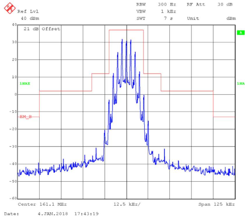
**FM,25kHz,Low Power - Frequency 161.1 MHz: 99% Occupied & 26 dB Bandwidth**
