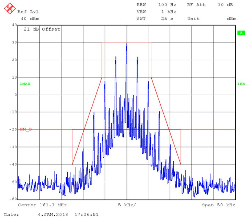
**FM,25kHz,High Power - Frequency 161.1 MHz: 99% Occupied & 26 dB Bandwidth**
