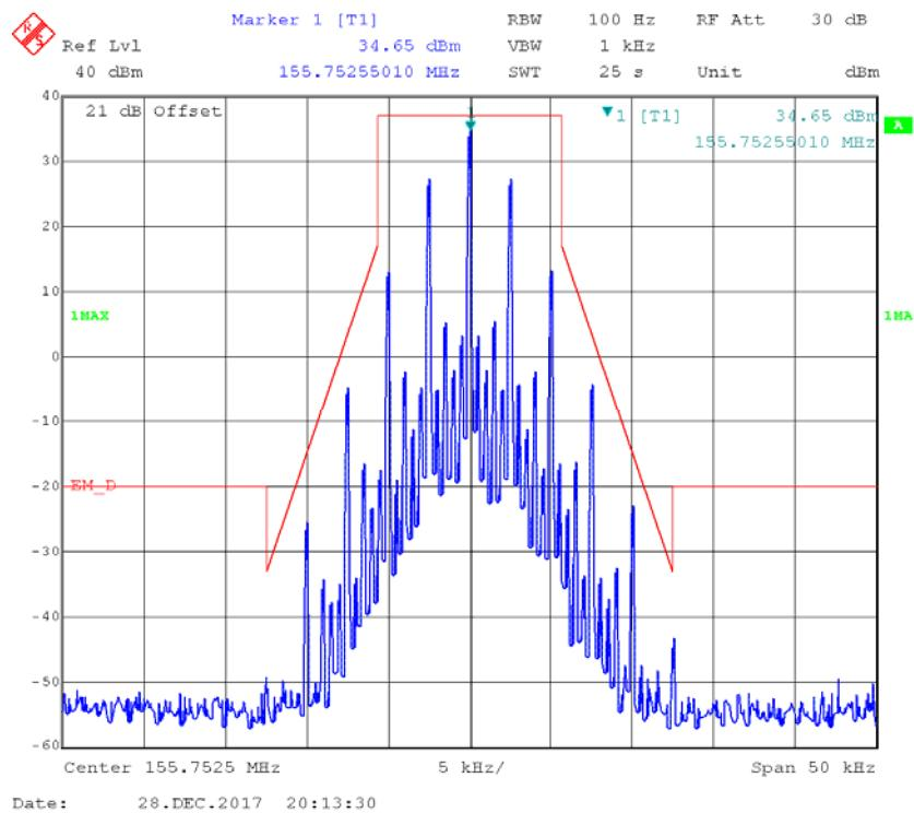
**FM,12.5kHz,Low Power - Frequency 155.7525 MHz: 99% Occupied & 26 dB Bandwidth**
