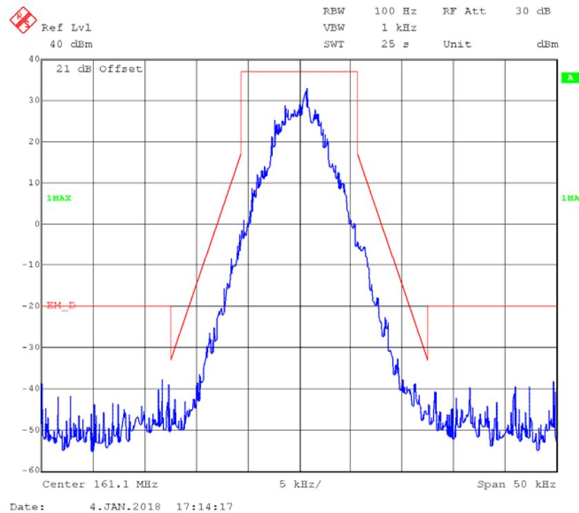
**4FSK,12.5kHz,Low Power - Frequency 161.1 MHz: 99% Occupied & 26 dB Bandwidth**
