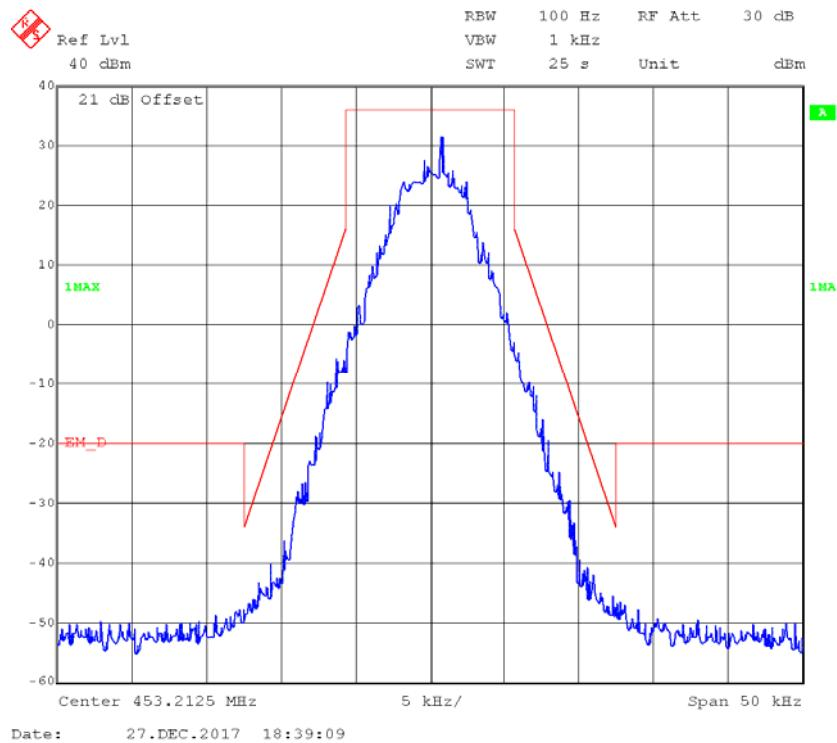
**4FSK,12.5kHz,Low Power - Frequency 453.2125 MHz: 99% Occupied & 26 dB Bandwidth**
