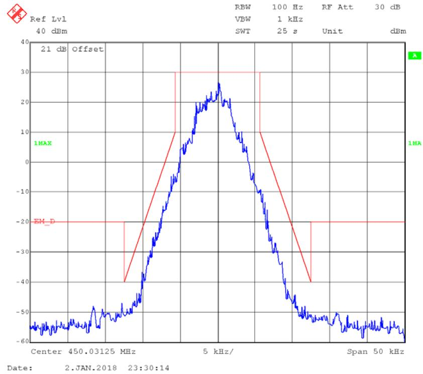
**Part 22:****FM,12.5kHz,High Power - Frequency 454.0125 MHz: 99% Occupied & 26 dB Bandwidth**
