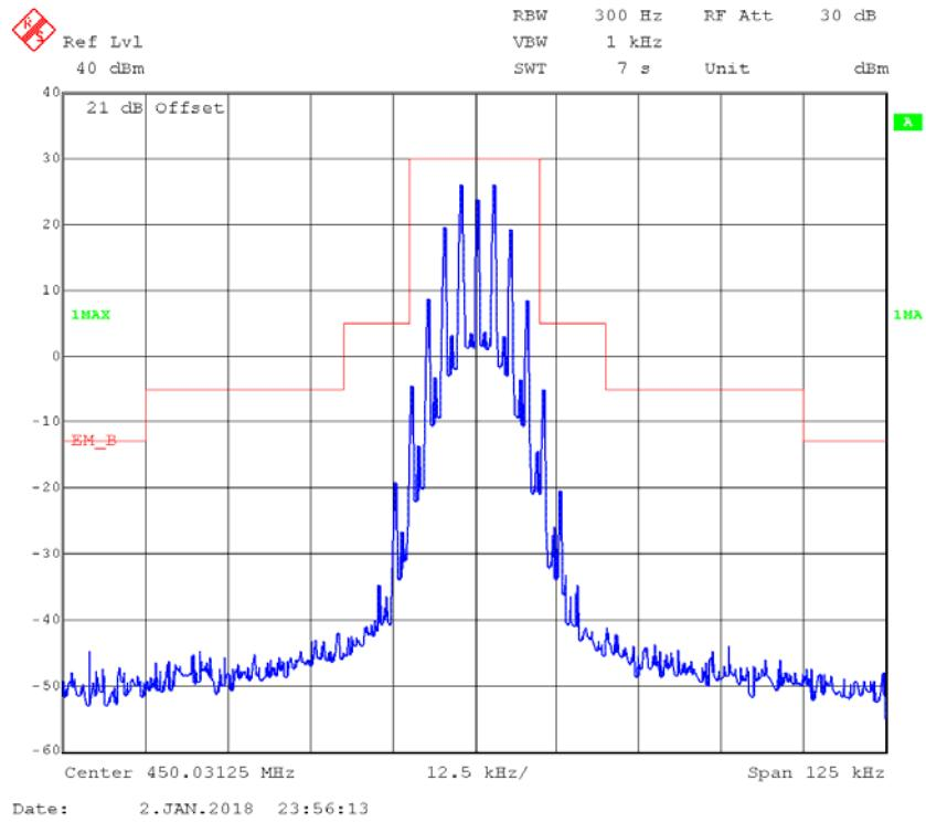
**4FSK,12.5kHz,High Power - Frequency 450.03125 MHz: 99% Occupied & 26 dB Bandwidth**
