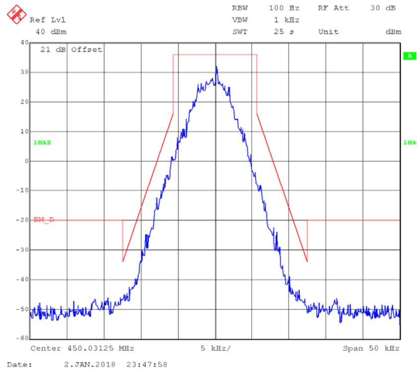
**4FSK,12.5kHz,Low Power - Frequency 450.03125 MHz: 99% Occupied & 26 dB Bandwidth**
