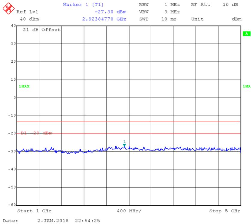
**12.5kHz, 4FSK, High power:****30MHz – 1 GHz, Channel Spacing 12.5 kHz, 450.03125 MHz**
