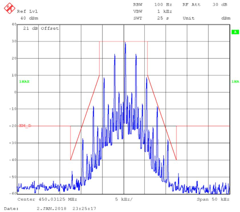
**FM,25kHz,High Power - Frequency 450.03125 MHz: 99% Occupied & 26 dB Bandwidth**
