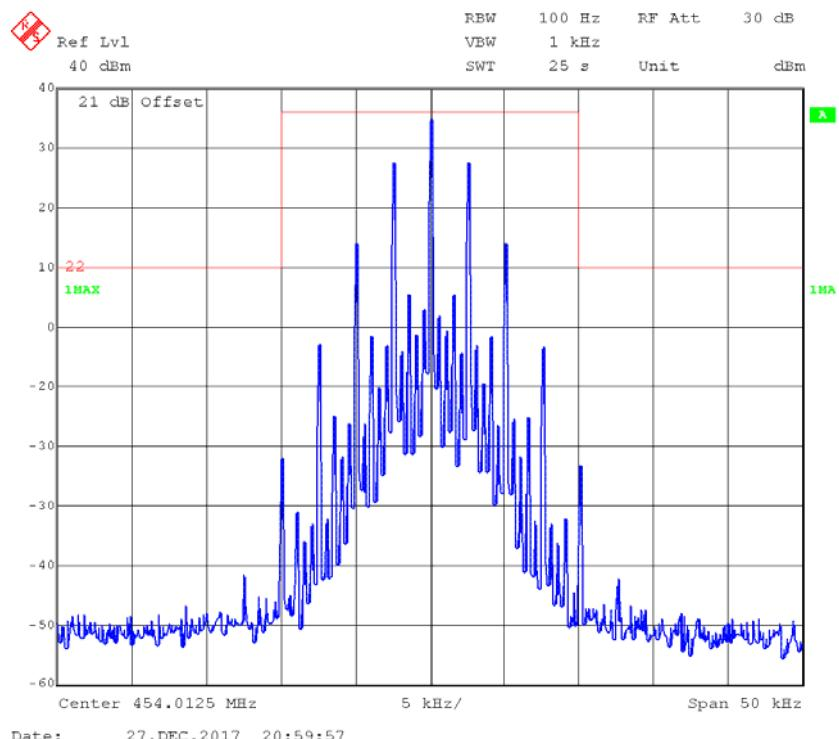
**FM,12.5kHz,Low Power - Frequency 454.0125 MHz: 99% Occupied & 26 dB Bandwidth**
