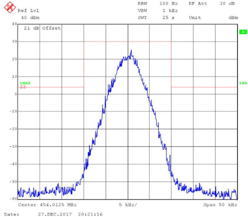
**FCC §2.1051 & §22.861 & §74.462 & § 80.211 & §90.210 - SPURIOUS EMISSIONS AT ANTENNA TERMINALS****Applicable Standard**
