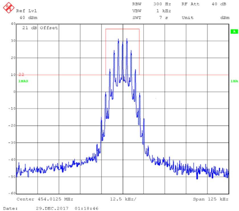
**FM,25kHz,Low Power - Frequency 454.0125 MHz: 99% Occupied & 26 dB Bandwidth**
