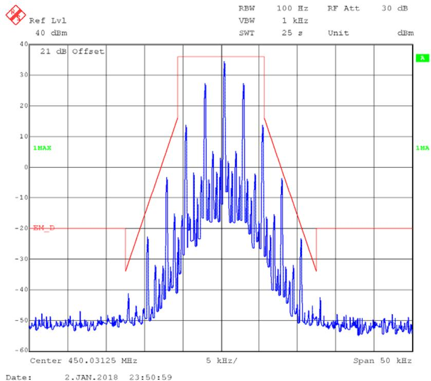
**FM,12.5kHz,Low Power - Frequency 450.03125 MHz: 99% Occupied & 26 dB Bandwidth**
