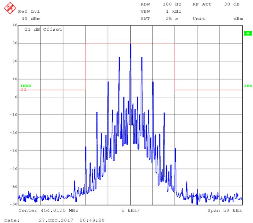
**FM,25kHz,High Power - Frequency 454.0125 MHz: 99% Occupied & 26 dB Bandwidth**
