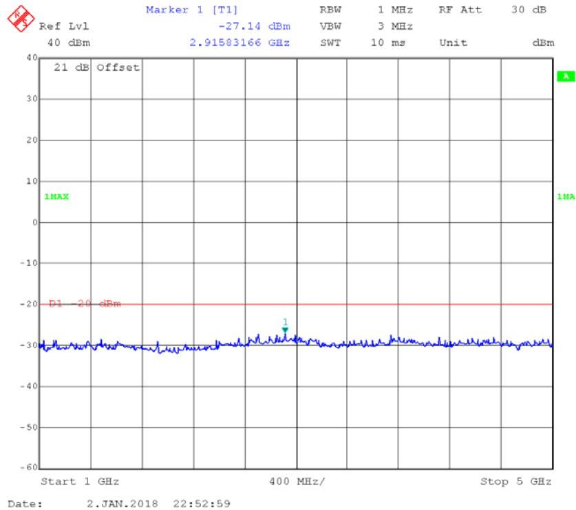
**25kHz, FM, High power(Emissions are under limit -13dBm):**
