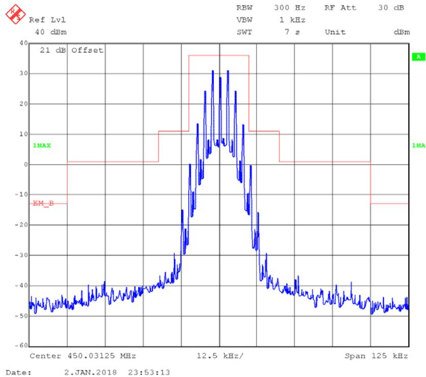
**FM,25kHz,Low Power - Frequency 450.03125 MHz: 99% Occupied & 26 dB Bandwidth**
