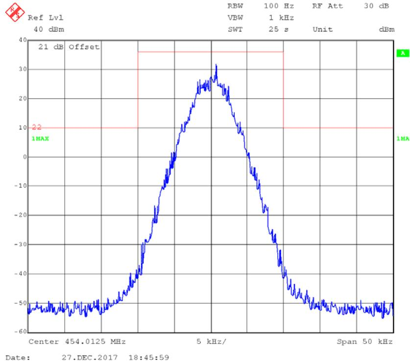
**4FSK,12.5kHz,Low Power - Frequency 454.0125 MHz: 99% Occupied & 26 dB Bandwidth**
