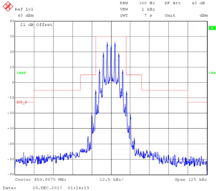
**Part 74:****FM,12.5kHz,High Power - Frequency 450.03125 MHz: 99% Occupied & 26 dB Bandwidth**
