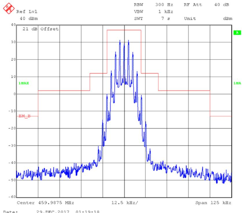
**FM,25kHz,Low Power - Frequency 459.9875 MHz MHz: 99% Occupied & 26 dB Bandwidth**
