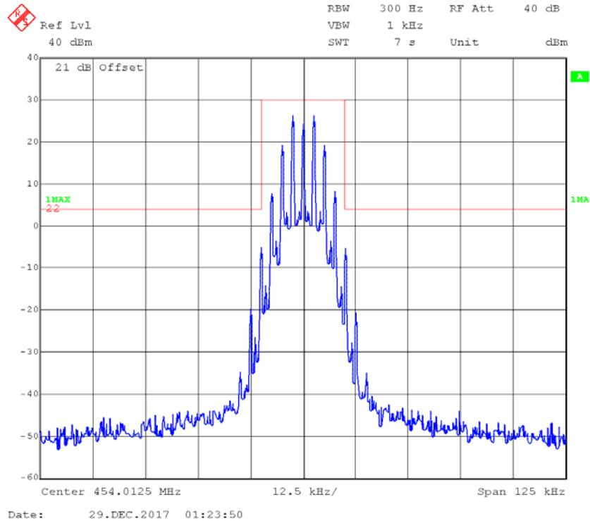
**4FSK,12.5kHz,High Power - Frequency 454.0125 MHz: 99% Occupied & 26 dB Bandwidth**
