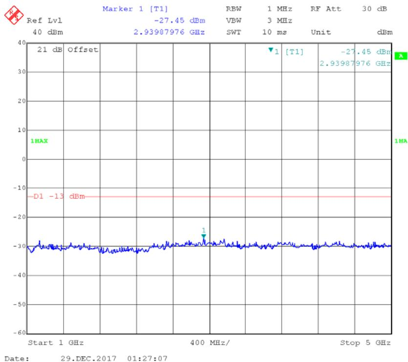
**12.5kHz, 4FSK, High power:****30MHz – 1 GHz, Channel Spacing 12.5 kHz, 454.0125 MHz**
