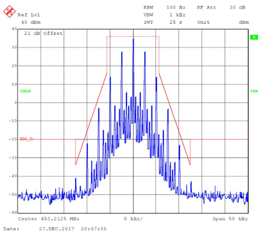
**FM,12.5kHz,Low Power - Frequency 453.2125 MHz: 99% Occupied & 26 dB Bandwidth**
