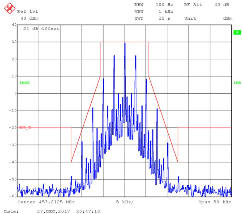
**4FSK,12.5kHz,High Power - Frequency 453.2125 MHz: 99% Occupied & 26 dB Bandwidth**
