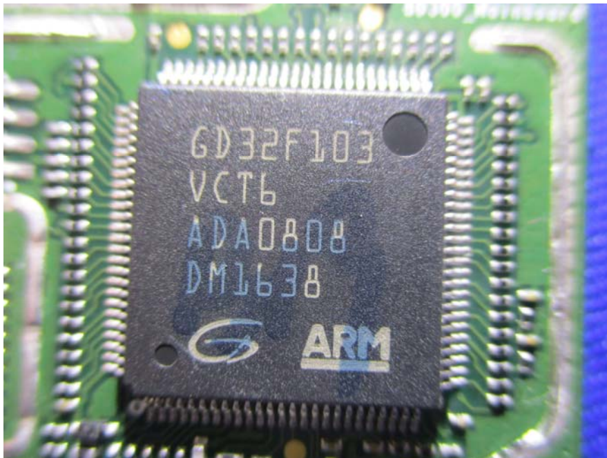
EUT –Main Chip View
