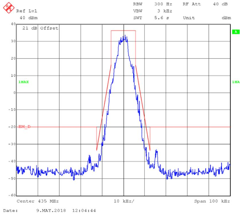
**4FSK,12.5kHz,Low Power - Frequency 435 MHz: 99% Occupied & 26 dB Bandwidth**
