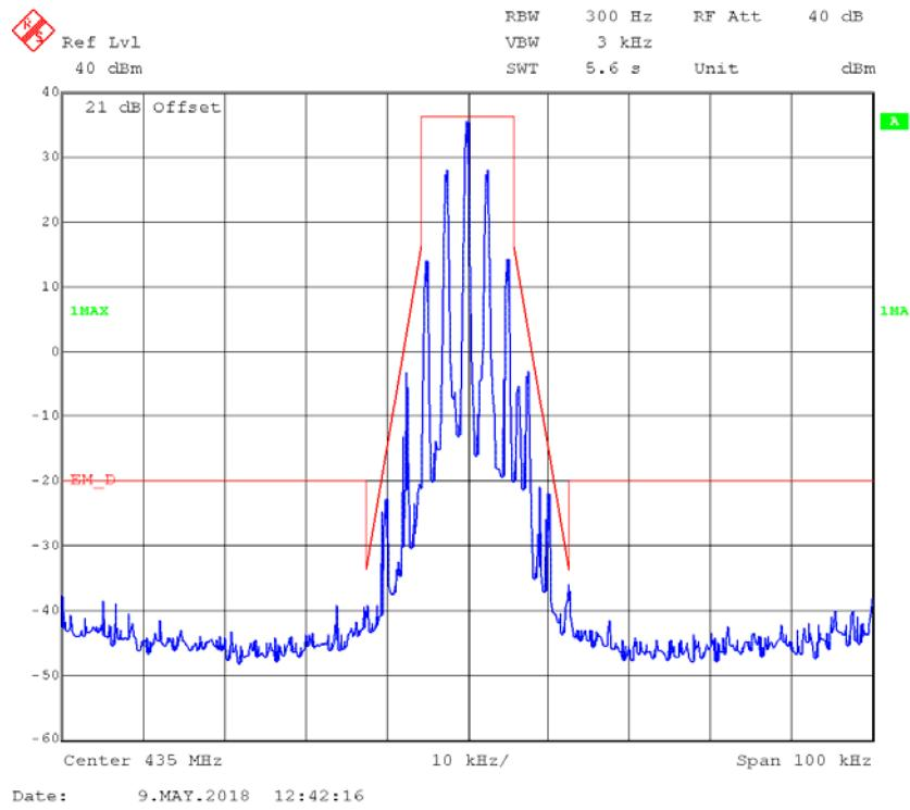
**FM,12.5kHz,Low Power - Frequency 435MHz: 99% Occupied & 26 dB Bandwidth**
