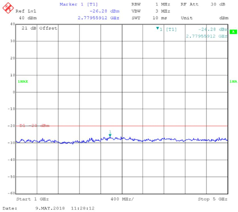
**12.5kHz, 4FSK, High power:****30MHz – 1 GHz, Channel Spacing 12.5 kHz, 435 MHz**
