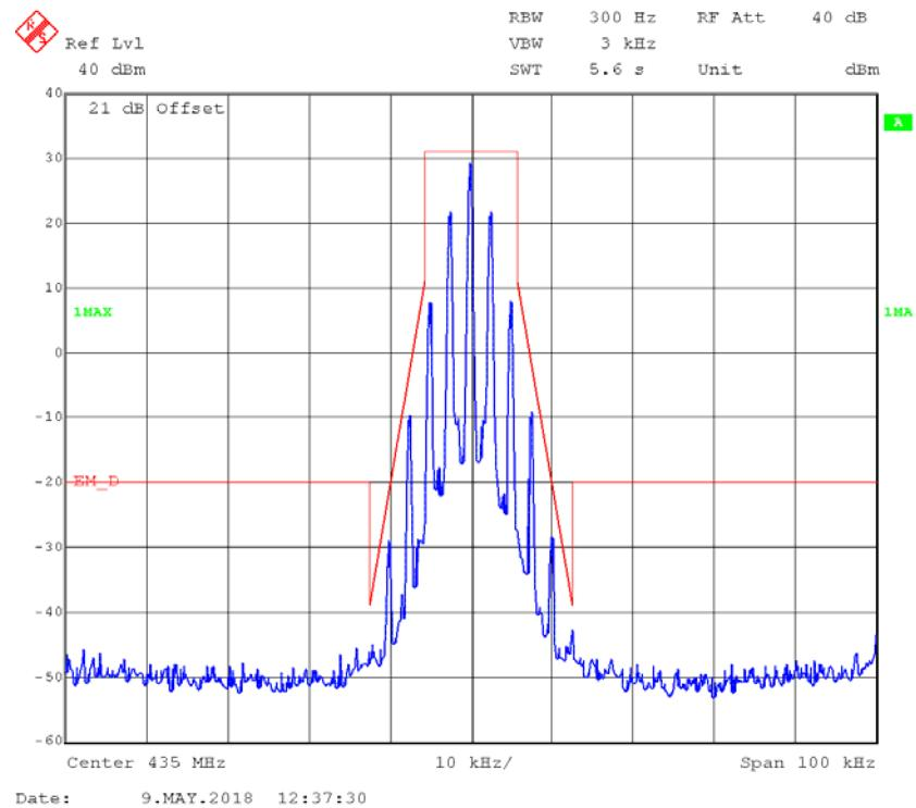
**4FSK,12.5kHz,High Power - Frequency 435 MHz: 99% Occupied & 26 dB Bandwidth**
