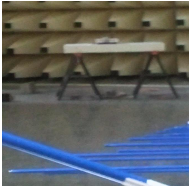
Figure 1: Radiated emissions setup below 1 GHz
