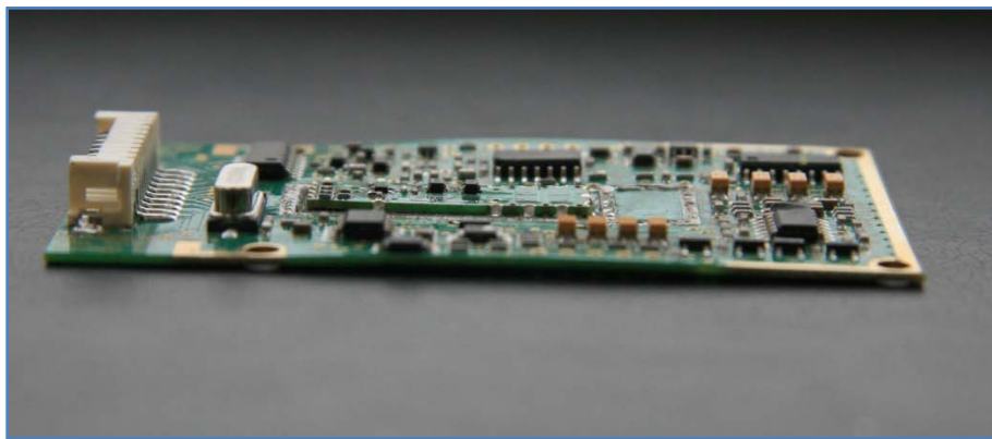
Figure 9: Sensor PCB, Side: Resonant Cavity Removed
