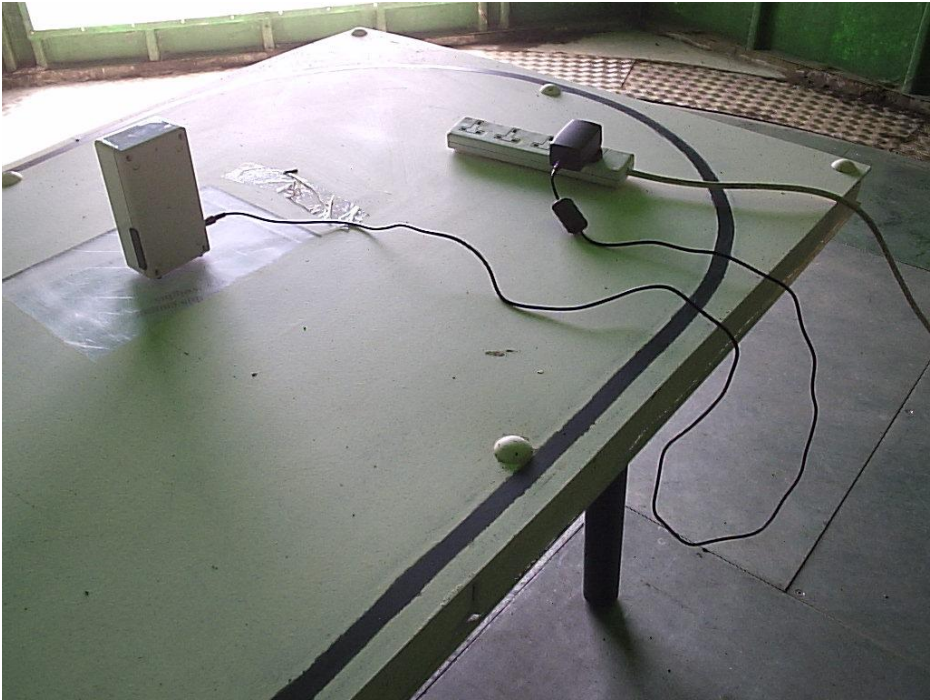
Figure 1: Radiated emissions setup on open area site
