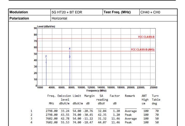
\*Factor includes antenna factor, cable loss and amplifier gain
