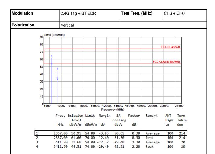
Note 1: Emission Level (dBuV/m) = SA Reading (dBuV/m) + Factor\* (dB) \*Factor includes antenna factor, cable loss and amplifier gain
