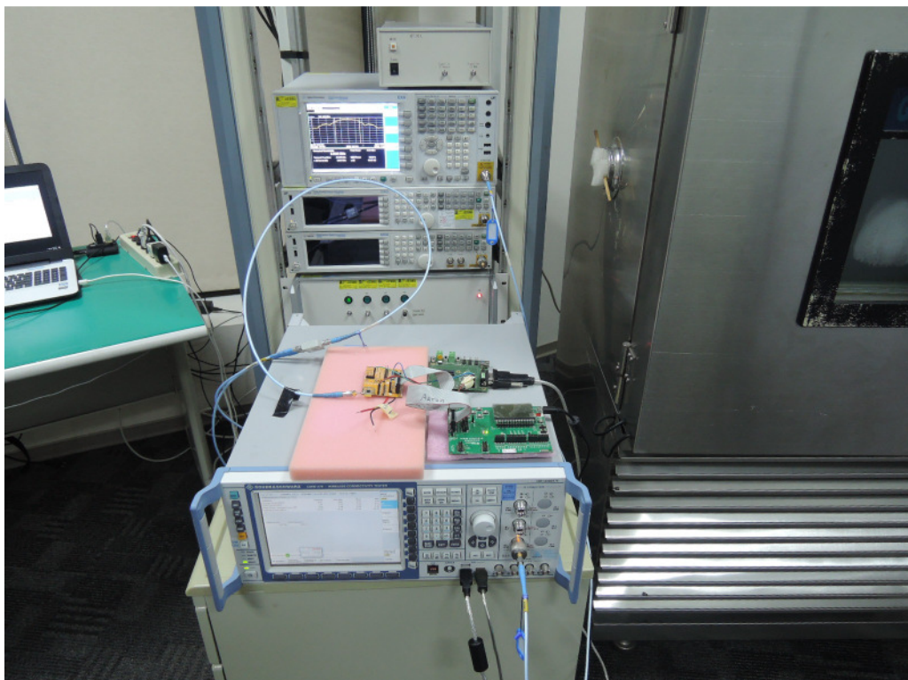
Photograph 5: Set-up for Conducted testing
