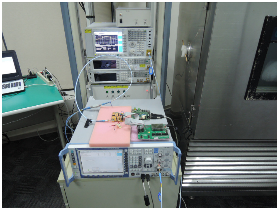
Photograph 5: Set-up for Conducted testing
