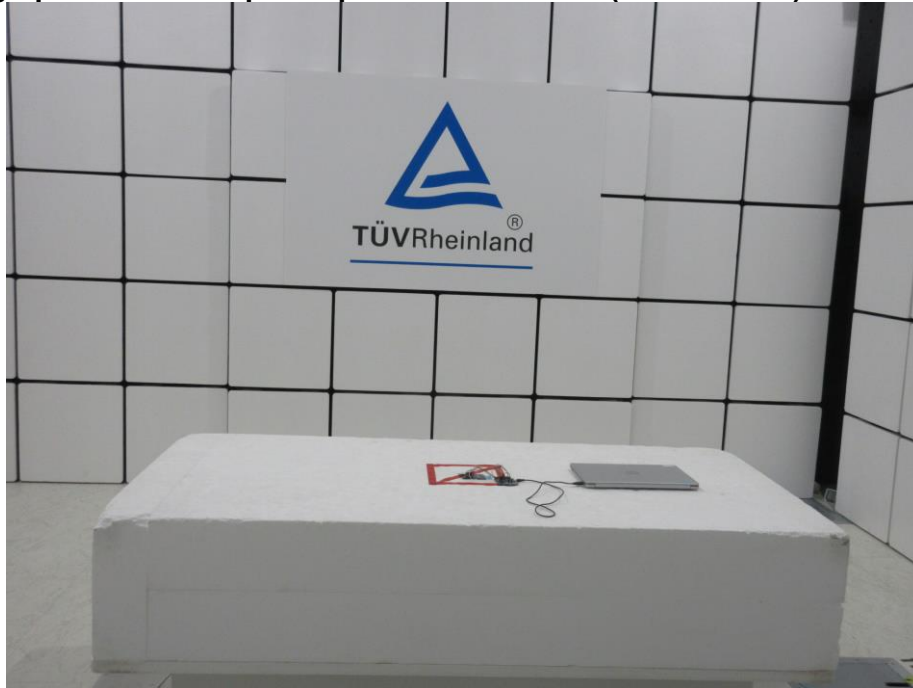
Photograph 2: Test Setup for Spurious Emissions (Front View 2)
