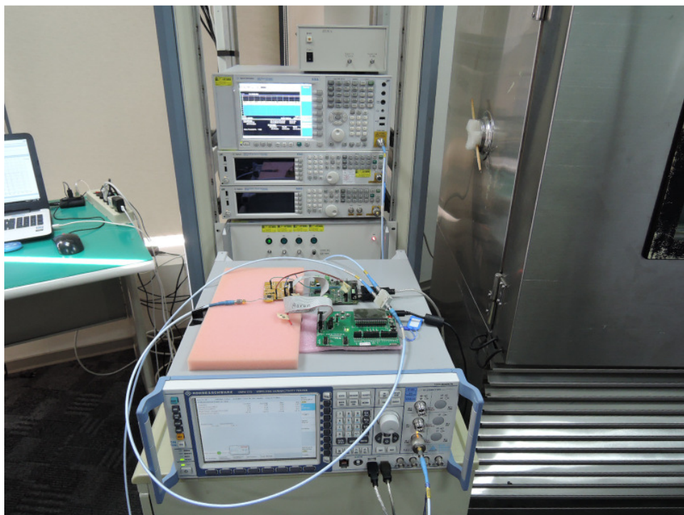
Photograph 5: Set-up for Conducted testing
