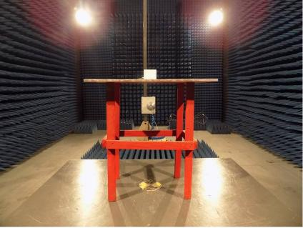
2 Photos of Band Edge Test (In Anechoic Chamber)
