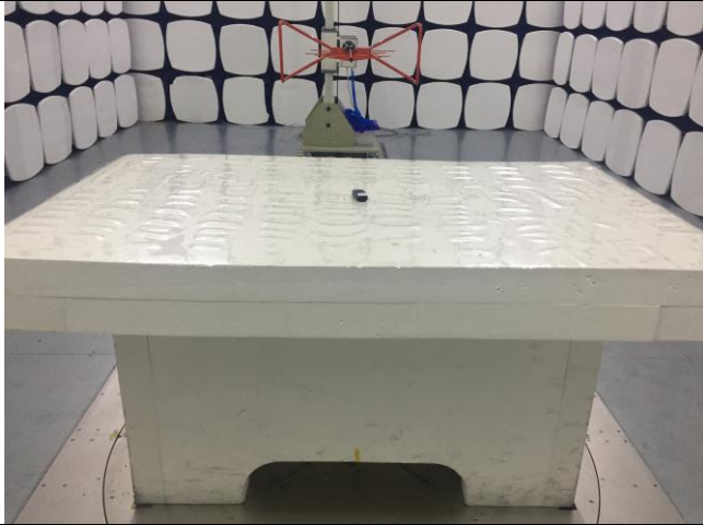
Radiated Spurious Emissions Test Setup Below 1GHz
