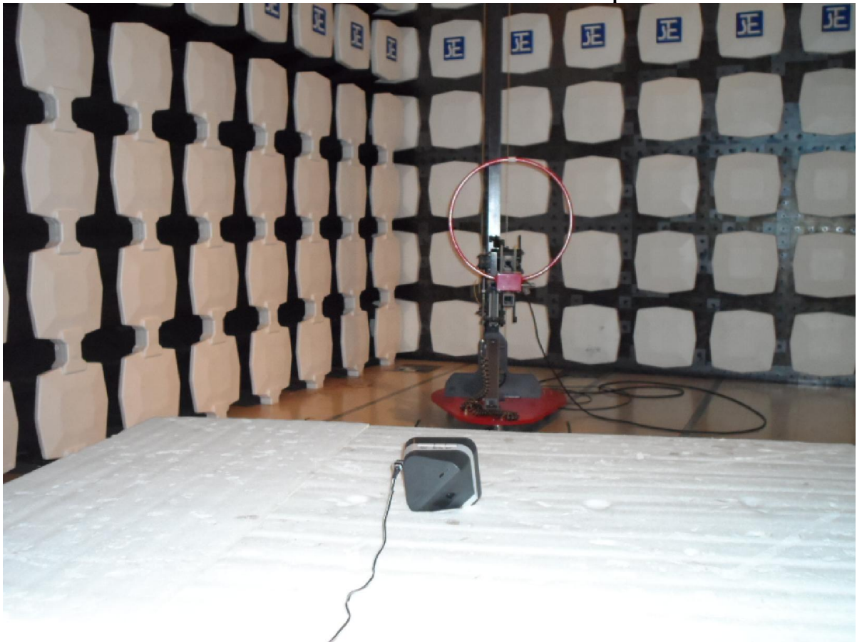
Measurement of Radiated Emission Test Set Up
