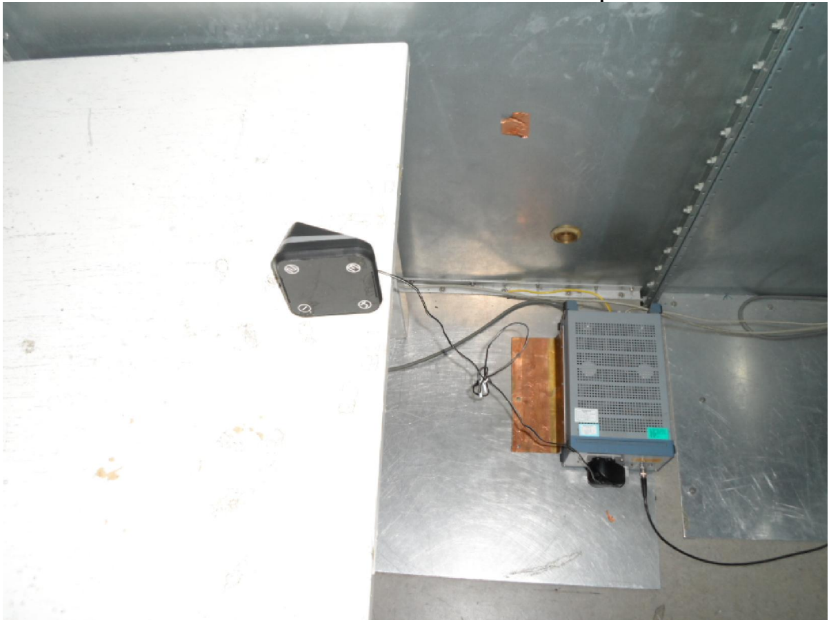
Measurement of Conducted Emission Test Set Up
