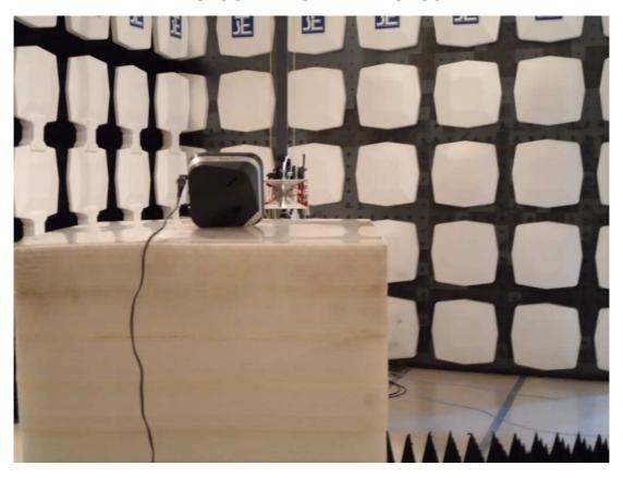
MEASUREMENT OF CONDUCTED EMISSION TEST SET UP
