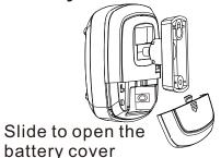
Insert a CR123A battery to the battery compartment.
