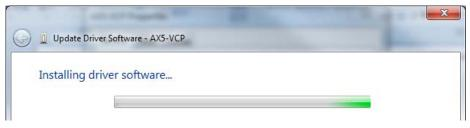
7. Once the installation is completed, you should be able to see the COM port showing. This will be the COM port you use for communicate with the AX7 when USB is plugged in.
