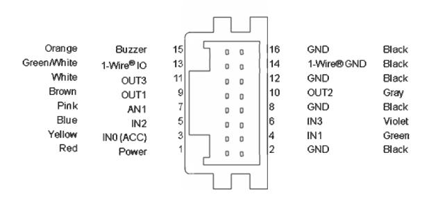
Positive Inputs: IN0, IN1 (Triggered when connects to V+ range from 3.7 ~ 40V)
