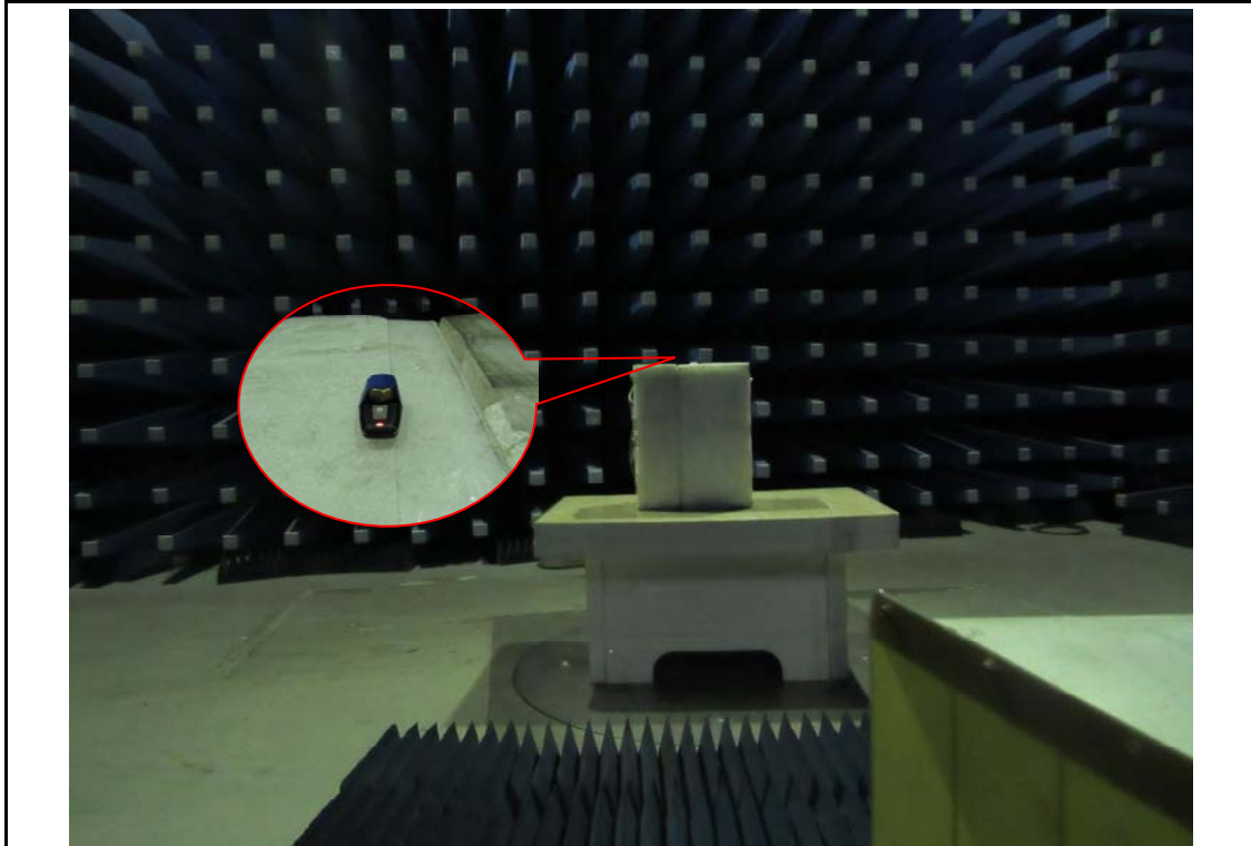
Radiated Spurious Emissions Test Setup Above 1GHz
