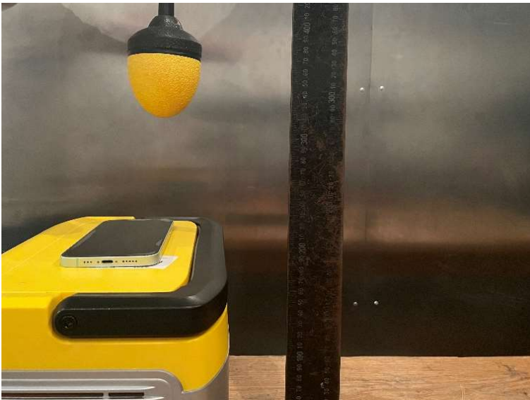
E-Field test (100kHz-3GHz at 20cm)
