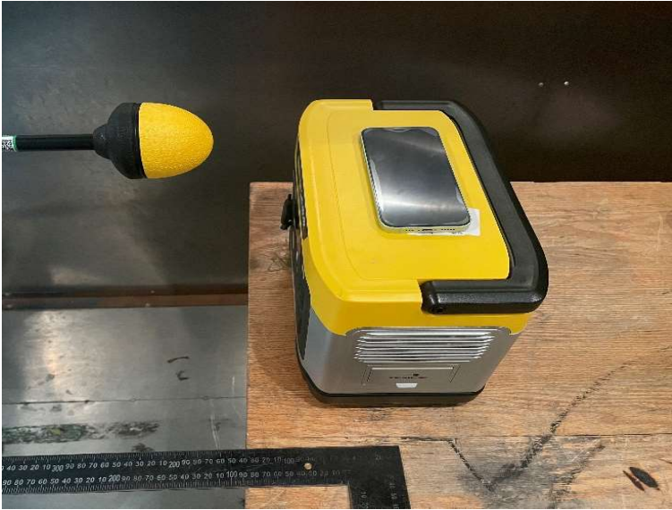
E-Field test (100kHz-3GHz at 15cm)
