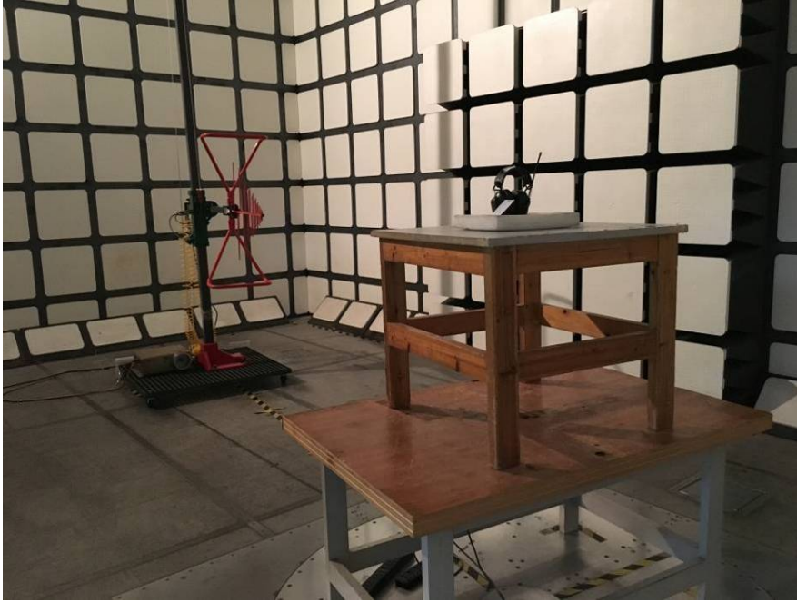
Radiated Emissions View (Below 1 GHz)
