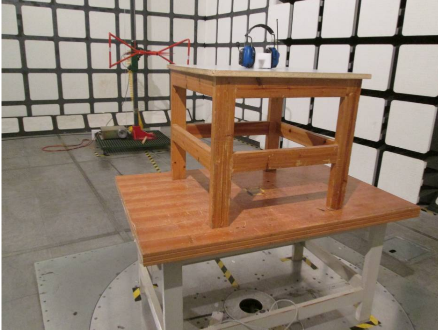
Radiated Emissions – Front View (Below 1 GHz)
