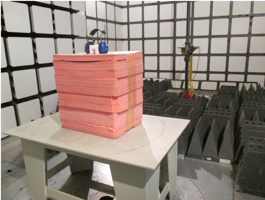
Radiated Emissions – Front View (Above 1 GHz)
