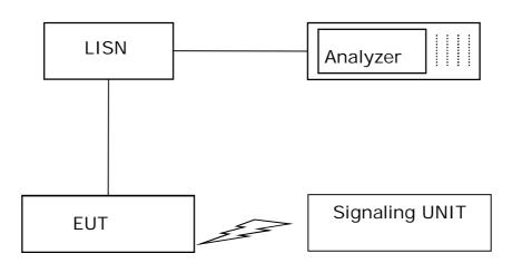
Setup in the shielded room for conducted measurements at AC mains port
